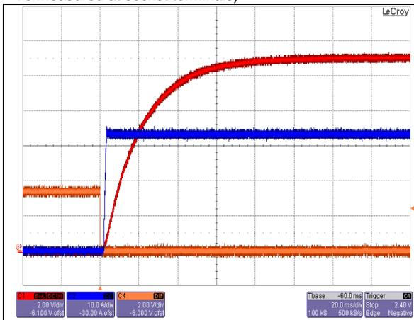
Start-up from on/off Switch at Vin,nom and Full Load.
