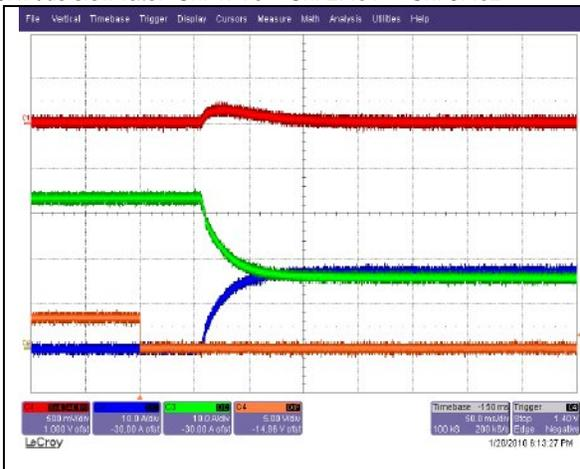
Start-up with back-biasing: Vin=48V, Io=33A
