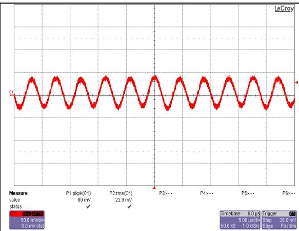
Typical Output Ripple at 48V Input and Full Load at Ta=25C
