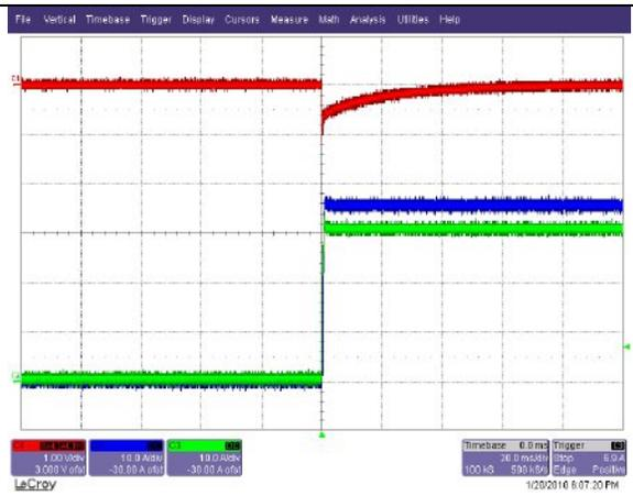
Load Transient Response. Load Step: 0A to 66A, 0.1A/us
