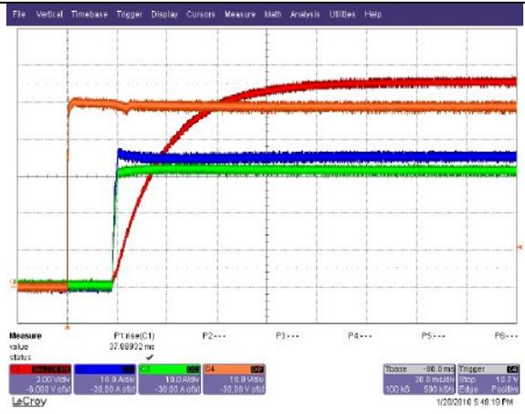
Start-up from Vin: 48Vin, Io=66A (200% Load)
