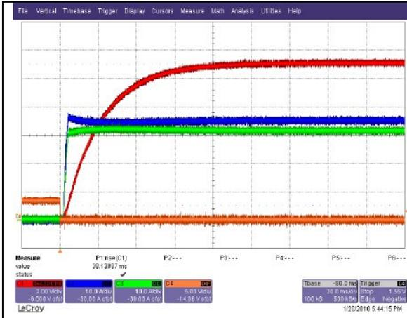
Start-up from on/off switch: 48Vin, Io=66A (200% Load)
