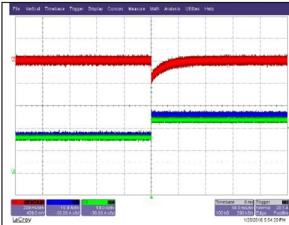
Load Transient Response. Load Step: 33A to 49.5A,
