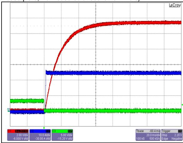
Start-up from on/off Switch at 48V input and Full Load.
