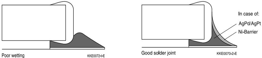
Good and poor solder joints caused by amount of solder in reflow soldering.
