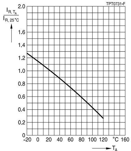
**Characteristics (typical) for  $T_{ref} = 120\text{ }^{\circ}\text{C}$**
