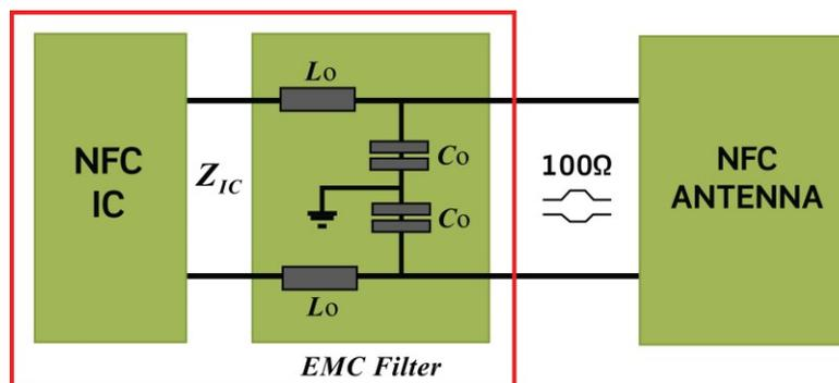
The matching circuit should be designed to match the IC impedance  $Z_{IC}$  to 100Ω and then connect the antenna through a 100Ω differential pair.
