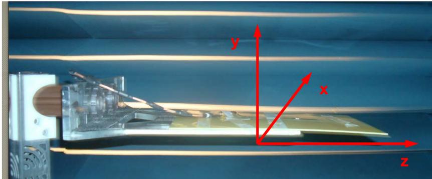
FXP831 on Baxter device to indicate the testing coordinate
