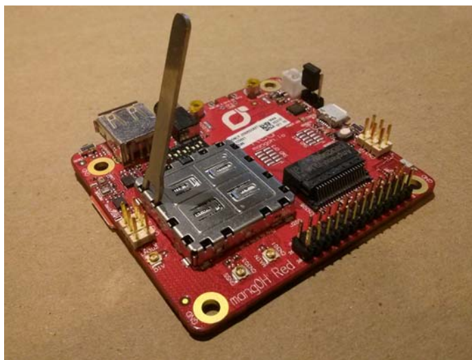
Figure 3-3: mangOH Red—Module Removal
