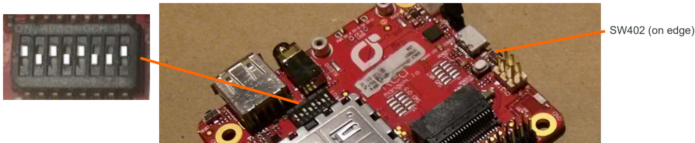
Figure 2-4: SW401 Dipswitch Recommended Settings
