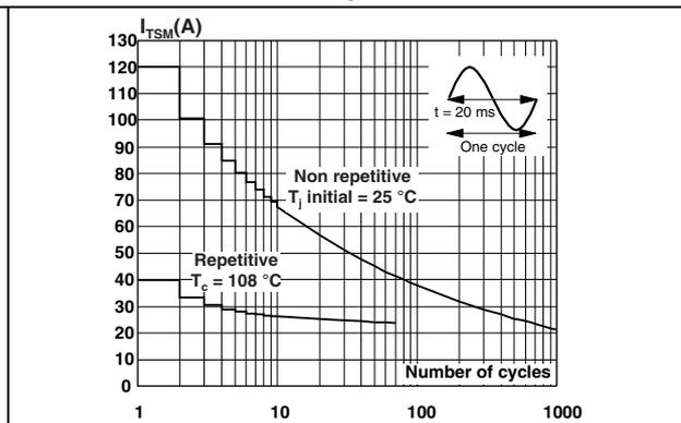
**Figure 7. Non repetitive surge peak on-state current and corresponding values of  $I^2t$**
