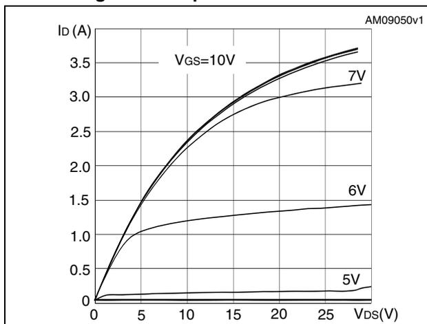
Figure 5. Transfer characteristics
