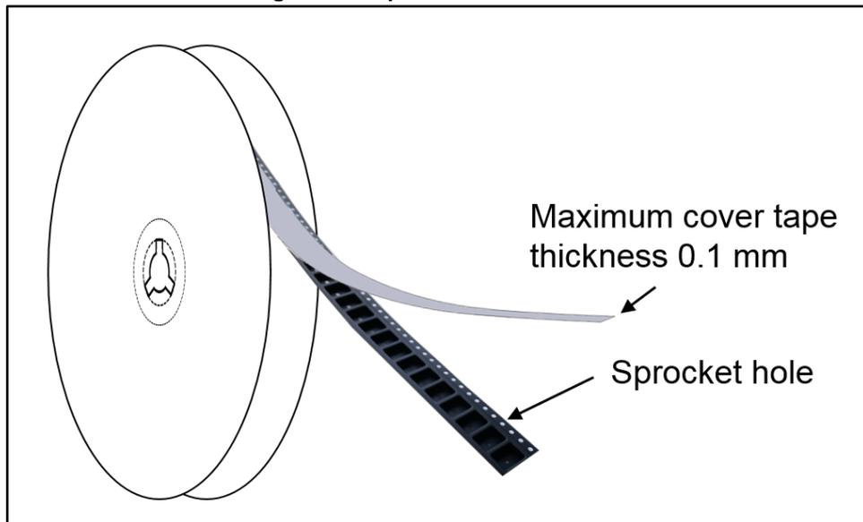
Figure 16: 13" Reel dimension definitions (mm)
