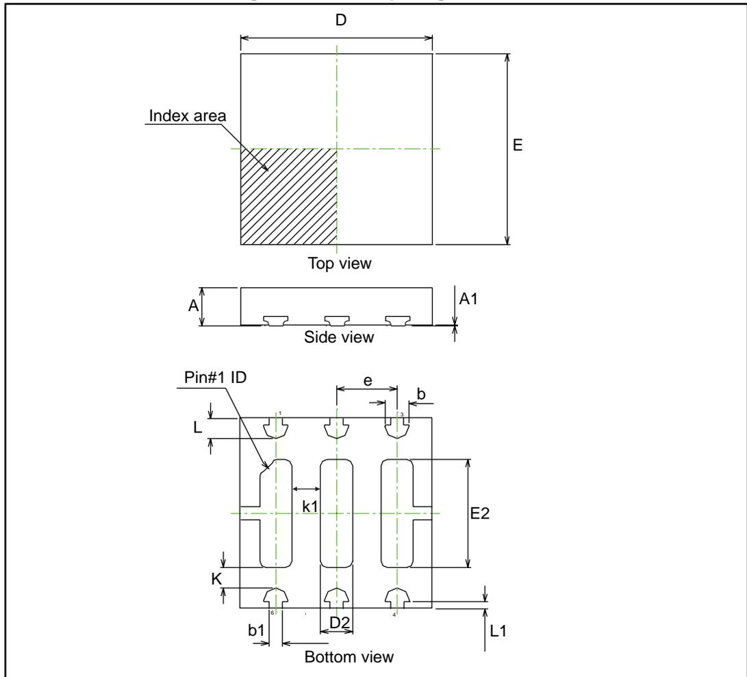
Table 7: QFN 3x3 package mechanical data
