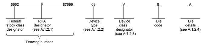
A.1.2.1 RHA designator. Device classes Q and V RHA identified die meet the MIL-PRF-38535 specified RHA levels. A dash (-) indicates a non-RHA die.
