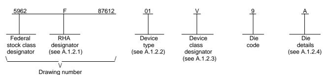
A.1.2.1 RHA designator. Device classes Q and V RHA identified die meet the MIL-PRF-38535 specified RHA levels. A dash (-) indicates a non-RHA die.
