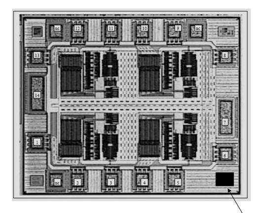
Pad size: Pad numbers 1 to 6 and 8 to 13: 100 x 100  $\mu$ m Pad numbers 7 (GND) and 14 (V<sub>CC</sub>): 100 x 280  $\mu$ m
