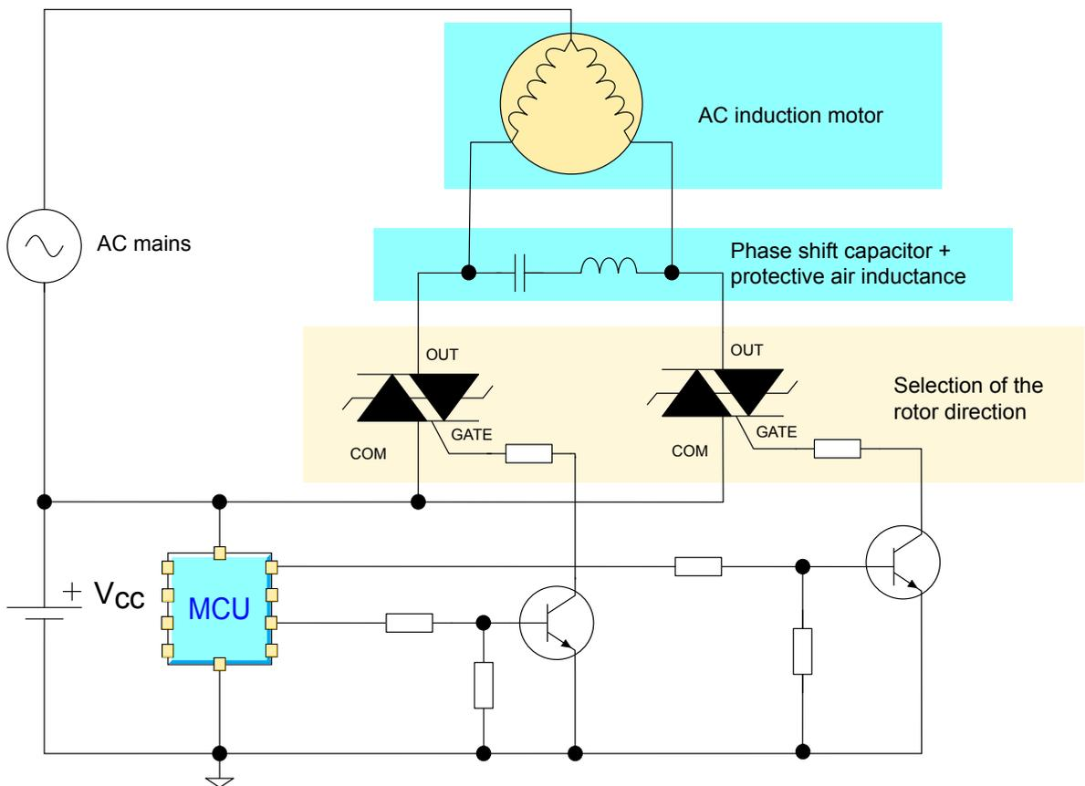
Figure 16. Universal drum motor control – typical diagram
