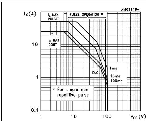
Figure 3. Derating curve
