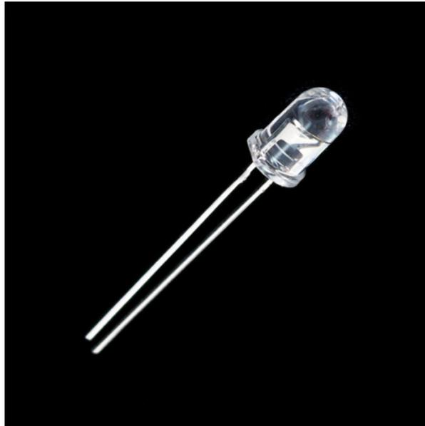
LED - Infrared 950nm
