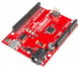
SparkFun RedBoard - Programmed with Arduino
