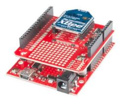
Part of what makes XBee so popular is its simplicity. XBees are controlled over a serial interface – in the most basic operation they can be used as a **wireless serial cable**. Setting up XBee networks and addresses is also simplified with Digi's free software – XCTU – which we explain in a separate tutorial.
