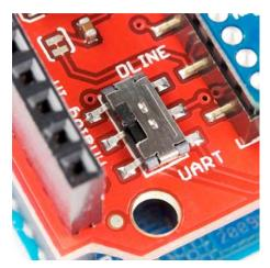
The Arduino Uno has a single hardware UART, which is usually either used for **programming** (via the Arduino's serial bootloader) or communication with the **serial monitor**. That serial port can only be used to communicate with one device at any time, lest you run into problems of bus contention. There's also a chance that, during program upload, spurious – even harmful – data might be sent to any device attached to the Arduino's hardware UART.
