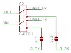
The switch configuration from the XBee Shield schematic. "D\_TX" connects to Arduino pin 3, and "D\_RX" connects to Arduino pin 2.
