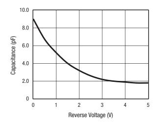
Figure 1. Capacitance vs Voltage
