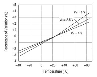
Figure 2. Relative Capacitance Change vs Temperature
