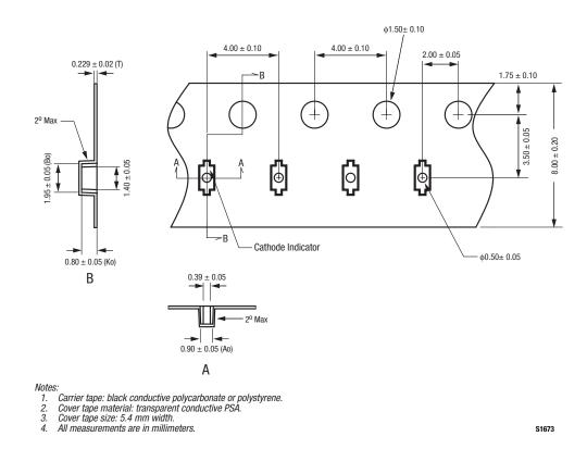
Figure 5. SC-79 Tape and Reel Dimensions
