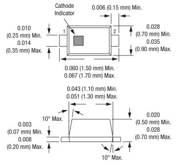
Dimensions are in inches (millimeters shown in parentheses) **\$1652**
