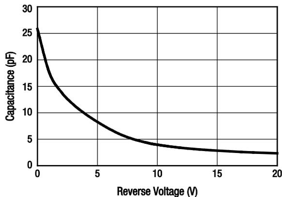
**Figure 1. Capacitance vs Reverse Voltage @ 25 °C**
