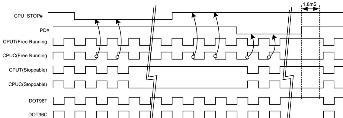
CPU\_STOP# = Driven, CPU\_PD = Driven, DOT\_PD = Driven
