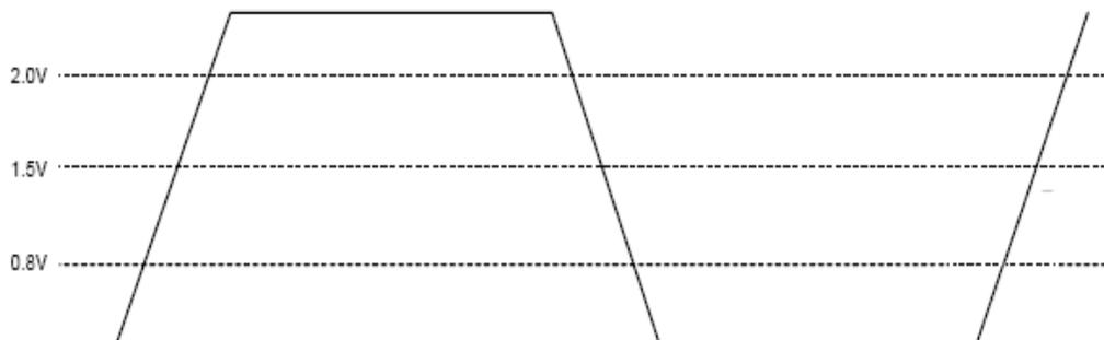
Figure 11. Single-ended Output Signals (for AC Parameters Measurement)
