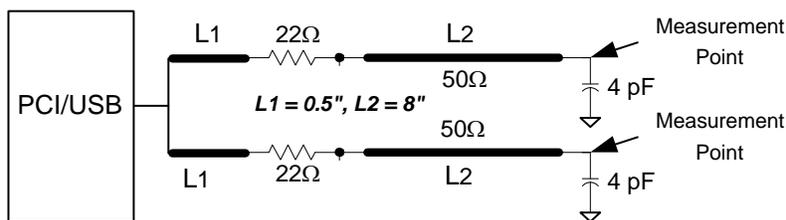
Figure 9. Single-ended PCI and USB Double Load Configuration
