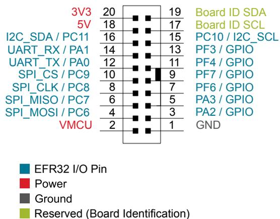
**Figure 4.3. Expansion Header**
