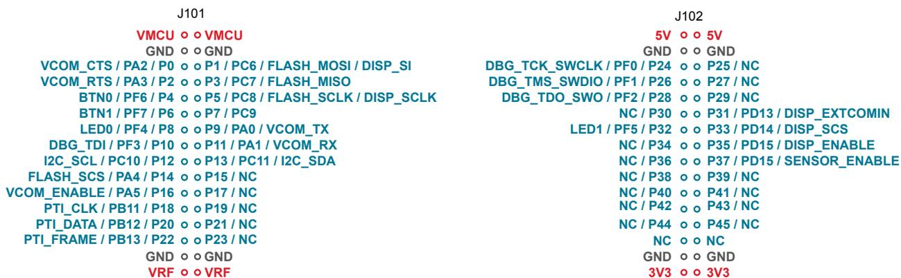
Figure 4.2. Radio Board Pin Mapping on Breakout Pads
