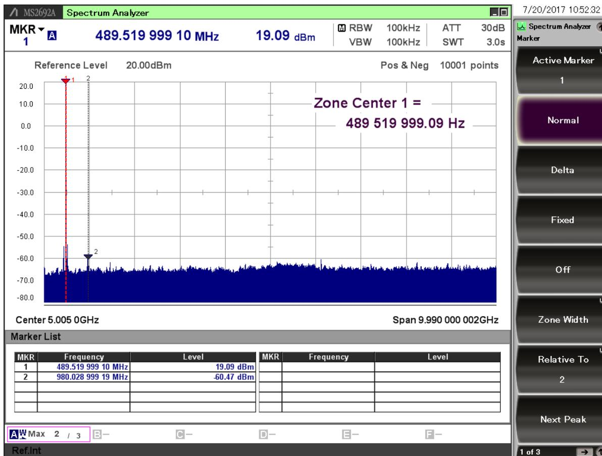
Figure 7.1. Typical Output Spectrum of the BRD4258A
