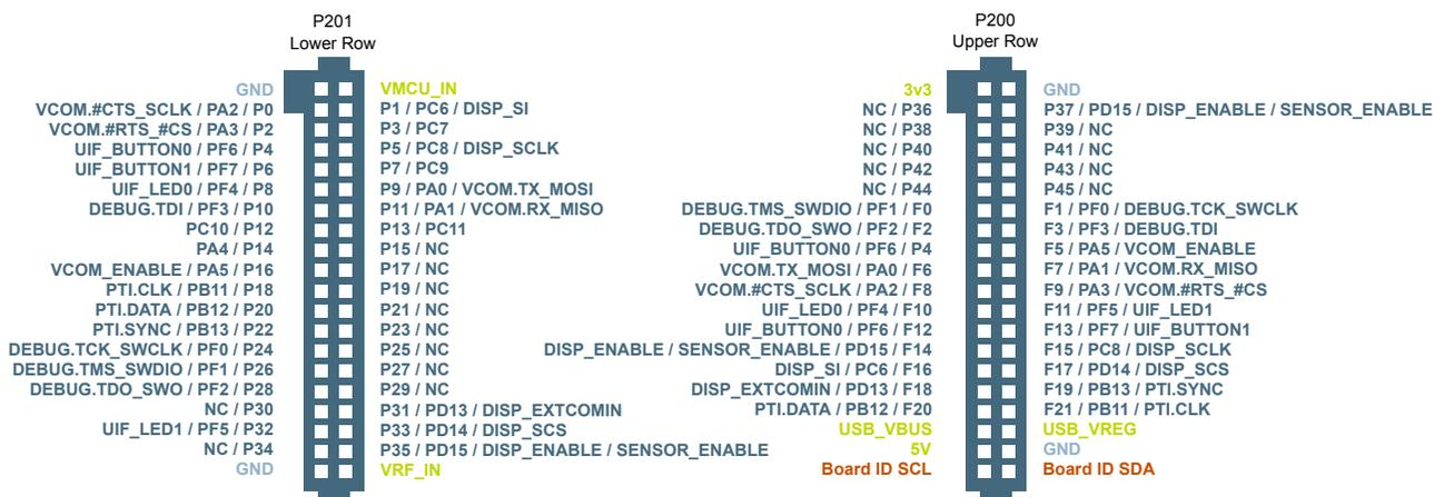
Figure 2.1. BRD4258A Radio Board Connector Pin Mapping
