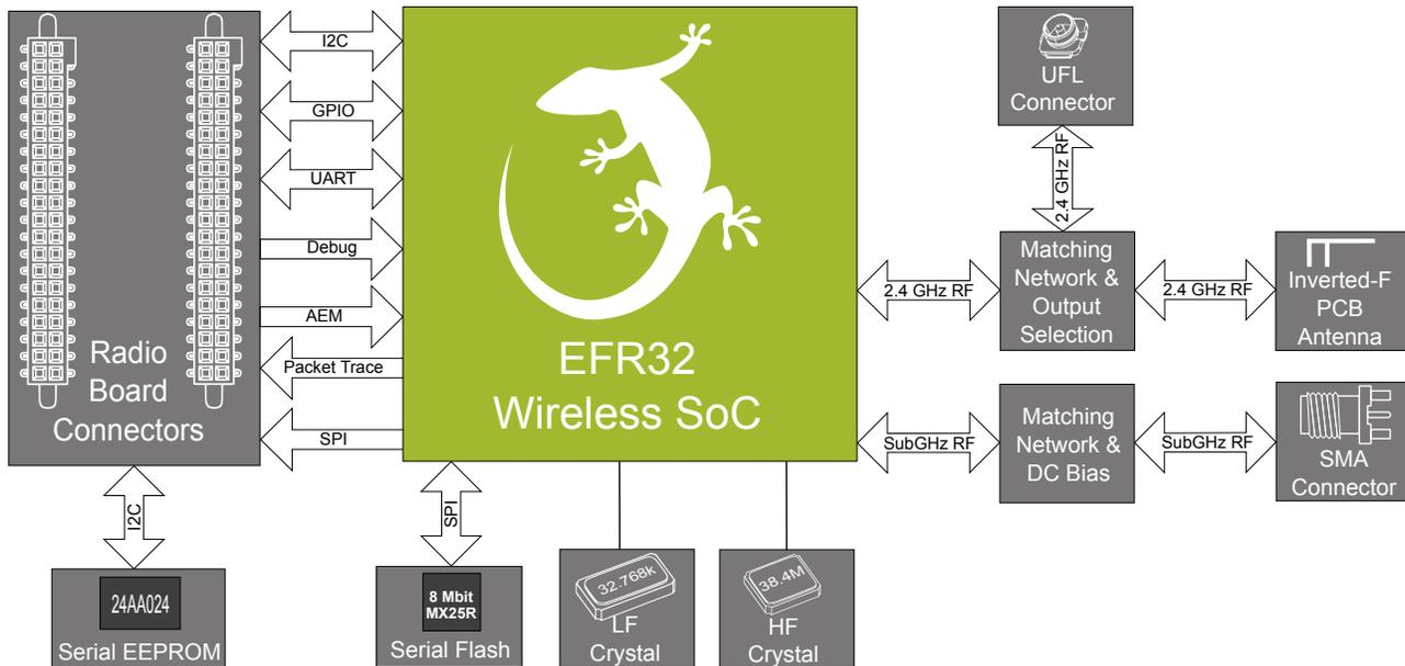
Figure 3.1. BRD4258A Block Diagram
