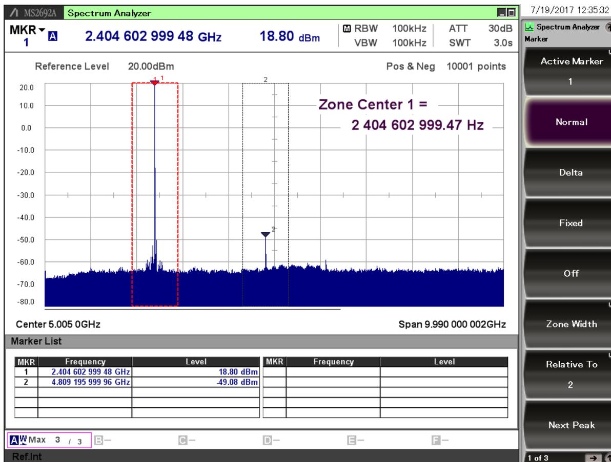
Figure 7.2. Typical Output Spectrum of the BRD4258A
