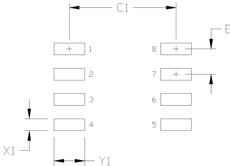
Figure 6.4. 8-Pin Narrow Body SOIC Land Pattern
