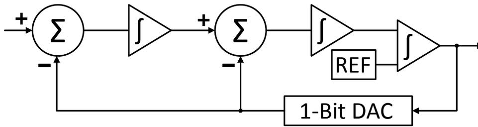
Figure 2.2. Typical 2nd Order Delta-Sigma Modulator Block Diagram
