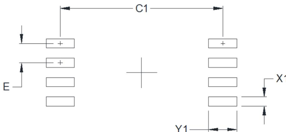
Figure 6.3. 8-Pin Wide Body Stretched SOIC Land Pattern
