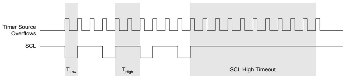
**Figure 24.4. Typical SMBus SCL Generation**
