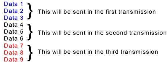
**Figure 23.13. Multiple Packets in TX Packet Handler**
