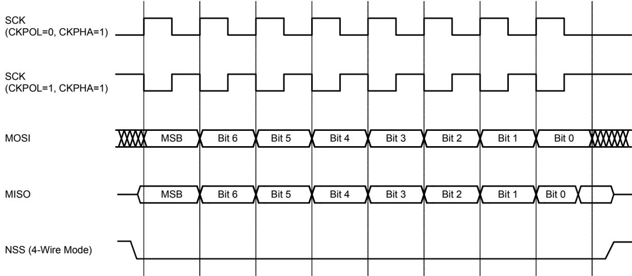
**Figure 26.7. Slave Mode Data/Clock Timing (CKPHA = 1)**
