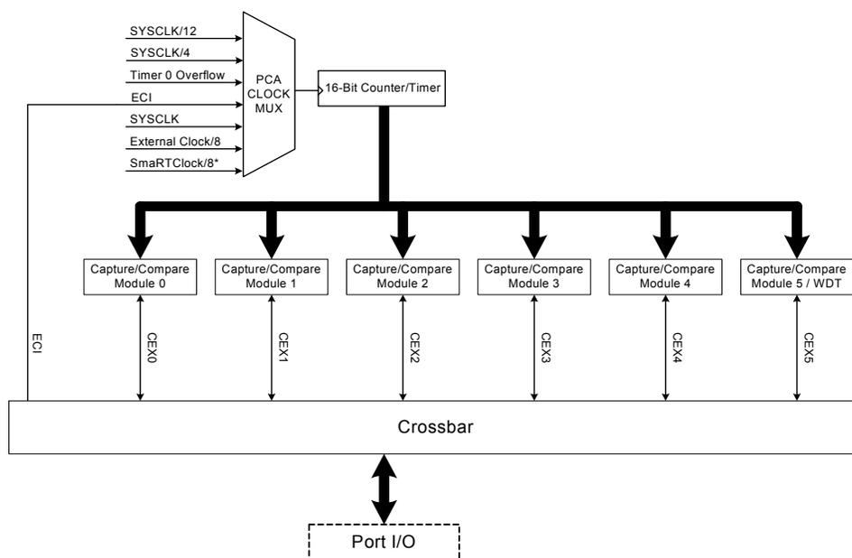
Figure 28.1. PCA Block Diagram
