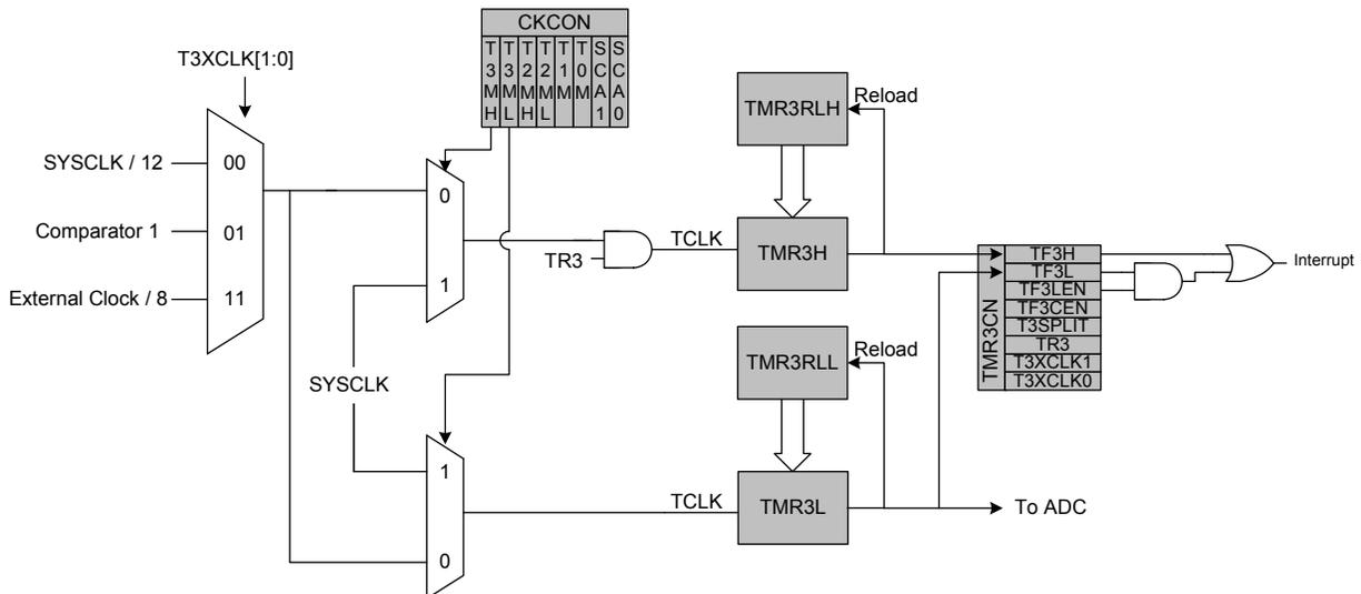
Figure 27.8. Timer 3 8-Bit Mode Block Diagram.
