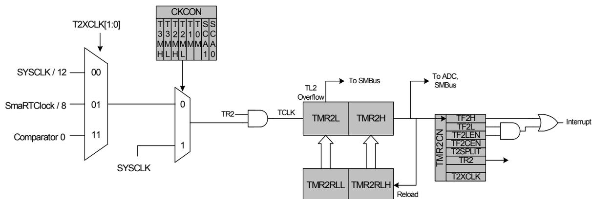
Figure 27.4. Timer 2 16-Bit Mode Block Diagram
