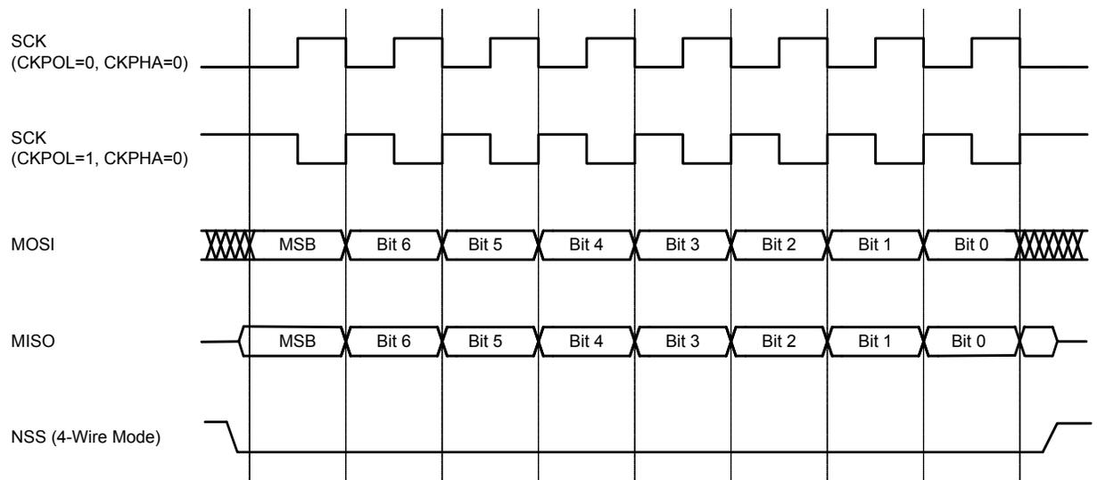
**Figure 26.6. Slave Mode Data/Clock Timing (CKPHA = 0)**
