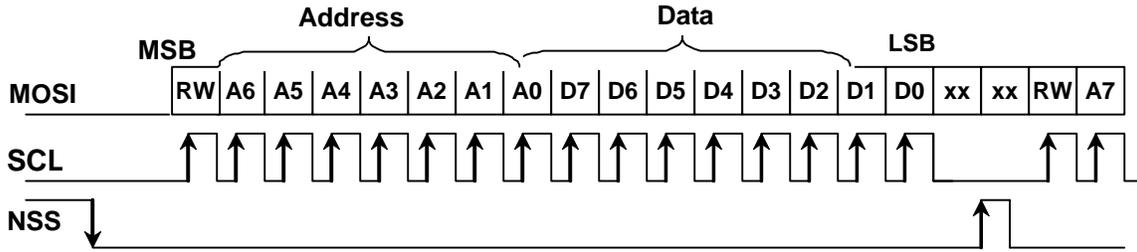
Figure 22.2. SPI Timing
