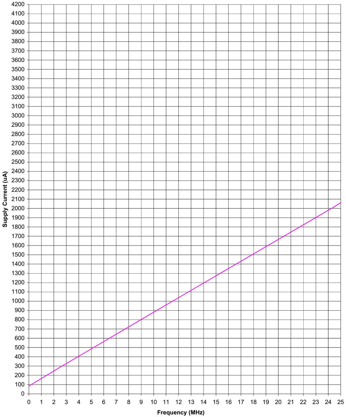
Figure 4.2. Idle Mode Current (External CMOS Clock)
