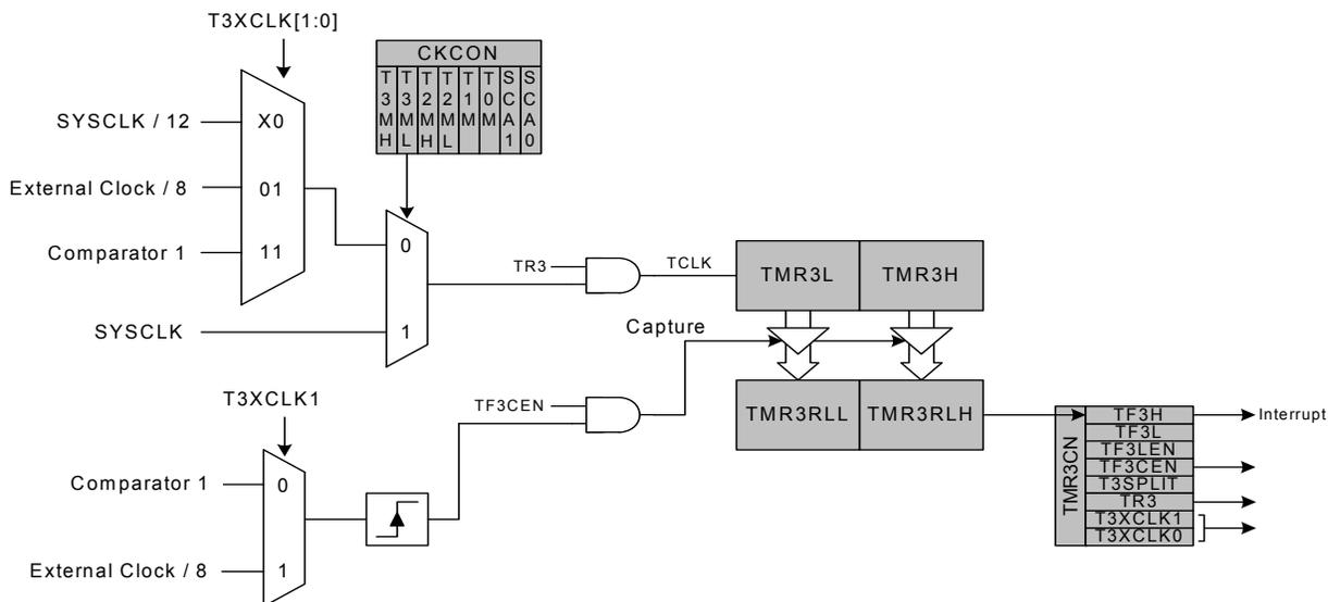
Figure 27.9. Timer 3 Capture Mode Block Diagram
