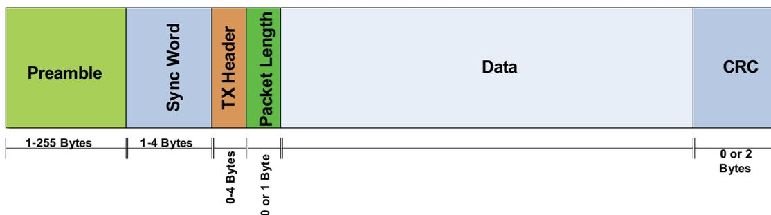
**Figure 23.12. Packet Structure**
