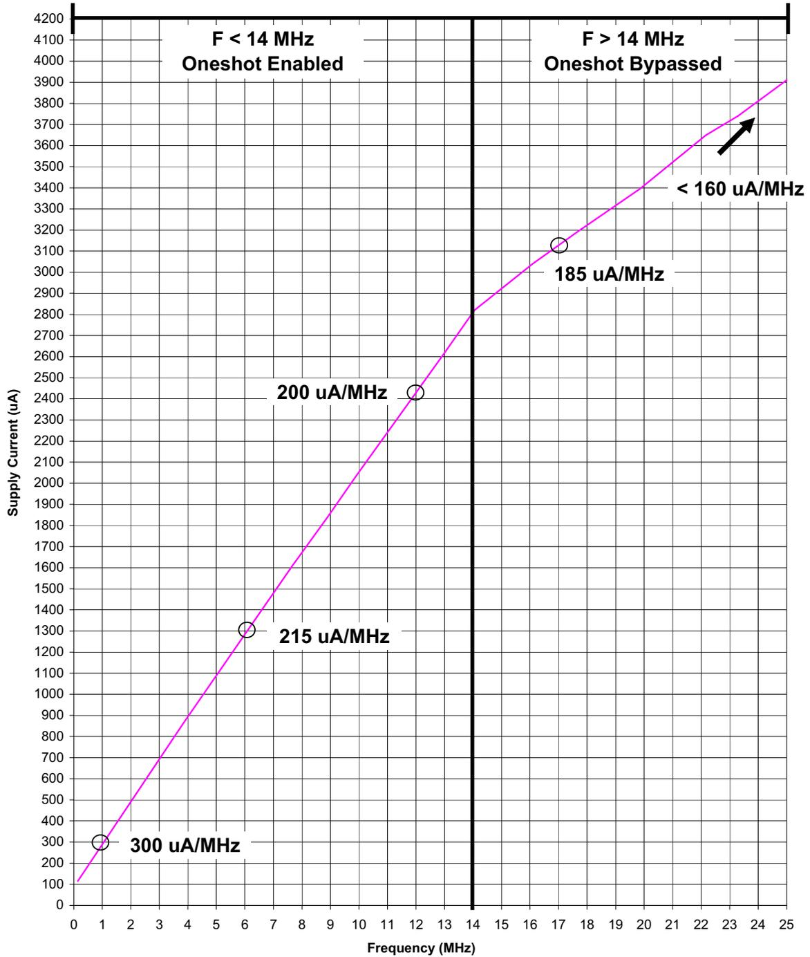
Figure 4.1. Active Mode Current (External CMOS Clock)
