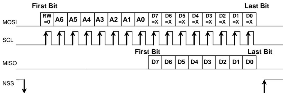
Figure 22.3. SPI Timing—READ Mode
