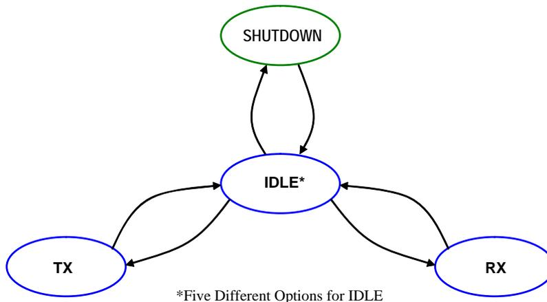
**Figure 23.1. State Machine Diagram**
