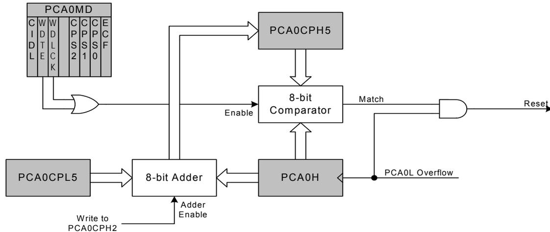
**Figure 28.11. PCA Module 5 with Watchdog Timer Enabled**
