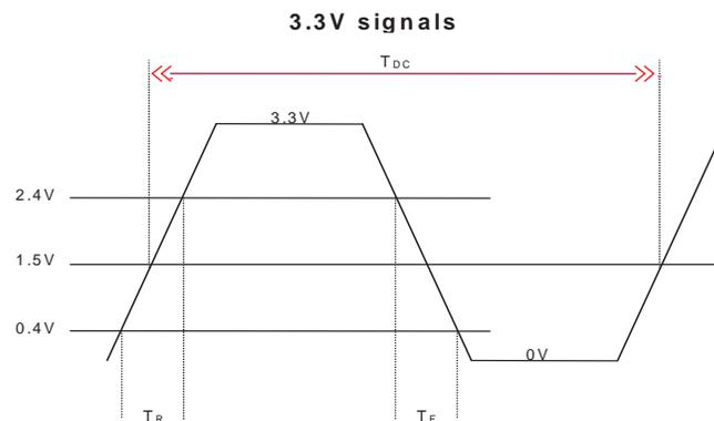
**Figure 6. Single-ended Output Signals (for AC Parameters Measurement)**
