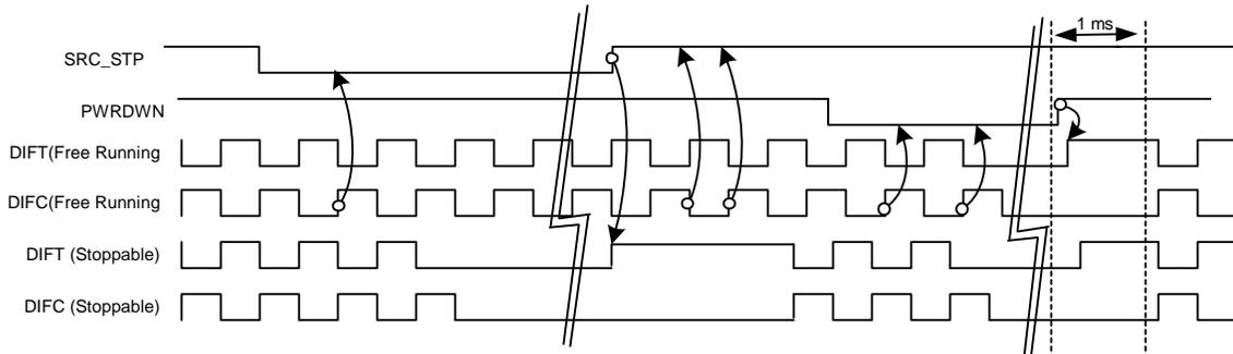
Figure 8. SRC\_STP = Tri-state, PWRDWN = Tri-state, OE\_INV = 0
