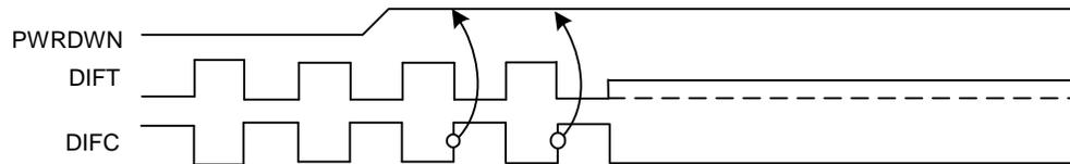
**Figure 2. PWRDWN Assertion Diagram, OE\_INV = 1**
