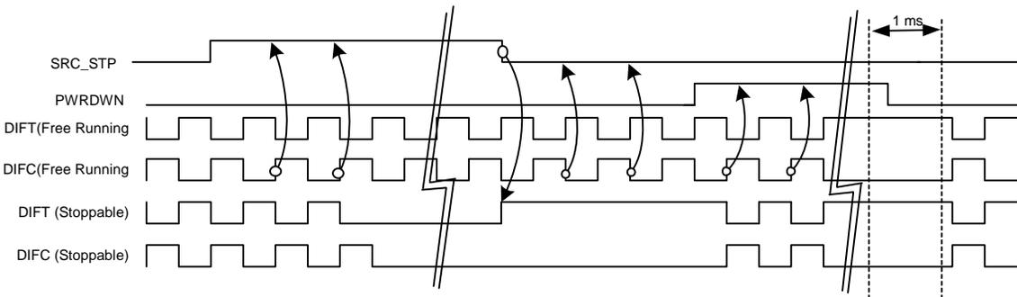
Figure 10. SRC\_STP = Tri-state, PWRDWN = Driven, OE\_INV = 1
