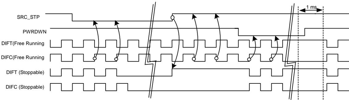
Figure 7. SRC\_STP = Tri-state, PWRDWN = Driven, OE\_INV = 0
