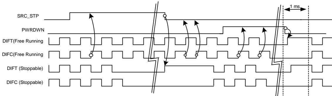
Figure 11. SRC\_STP = Tri-state, PWRDWN = Tri-state, OE\_INV = 1
