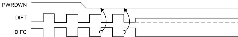
**Figure 1. PWRDWN Assertion Diagram, OE\_INV = 0**
