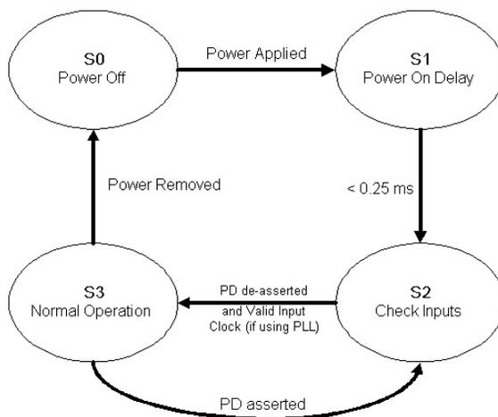
Figure 5. Buffer Power-up State Diagram<sup>[1]</sup>
