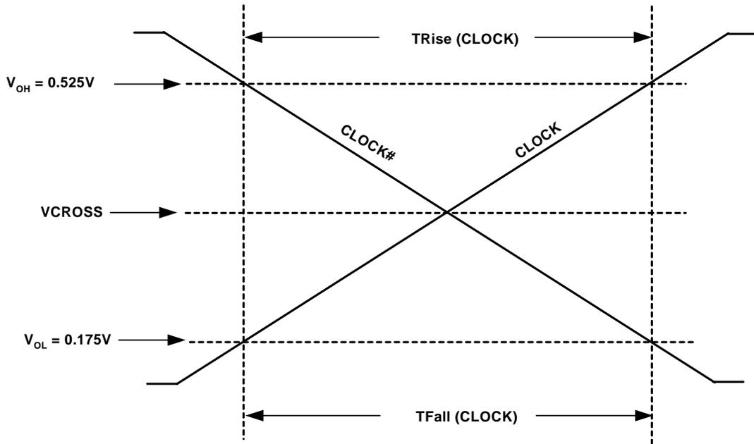
Figure 13. Single-Ended Measurement Points for TRise and TFall
