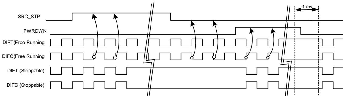
Figure 9. SRC\_STP = Driven, PWRDWN = Driven, OE\_INV = 1
