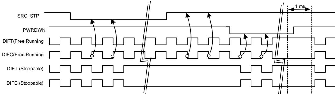
Figure 6. SRC\_STP = Driven, PWRDWN = Driven, OE\_INV = 0
