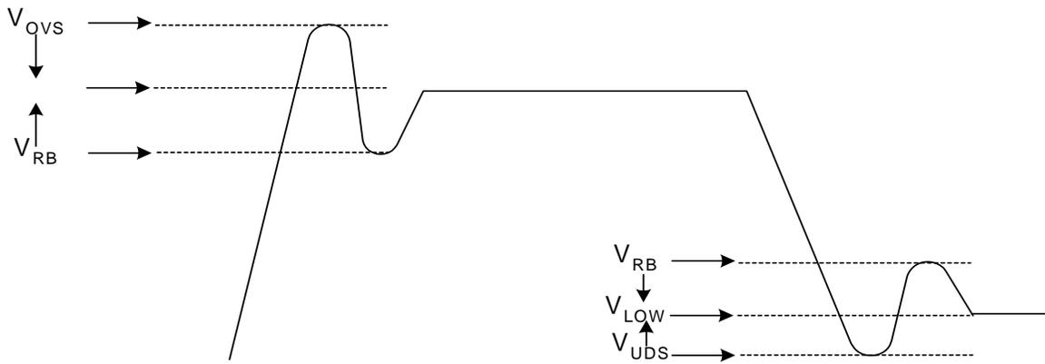
Figure 14. Single-ended Measurement Points for V<sub>OVS</sub>, V<sub>UDS</sub> and V<sub>RB</sub>
