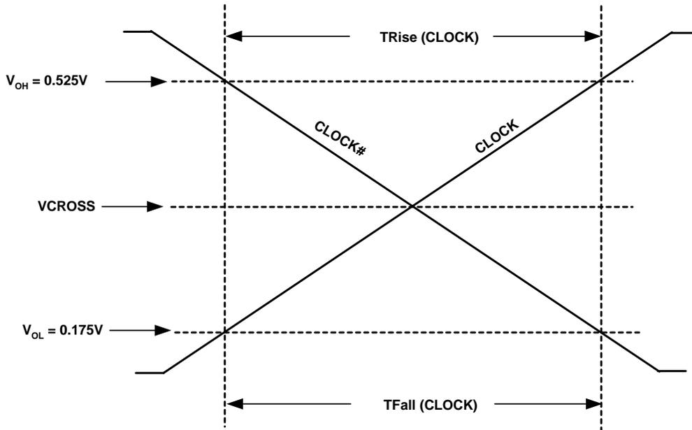
Figure 9. Single-Ended Measurement Points for TRise and TFall
