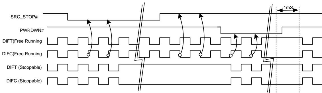
Figure 4. SRC\_STOP# = Driven, PWRDWN# = Driven
