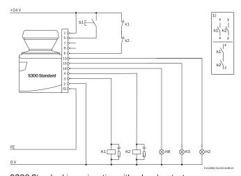
${\tt S300} \ Standard \ in \ conjunction \ with \ relays/contactors$
