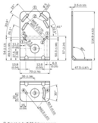
① Fixing hole for Dx50 distance sensors
