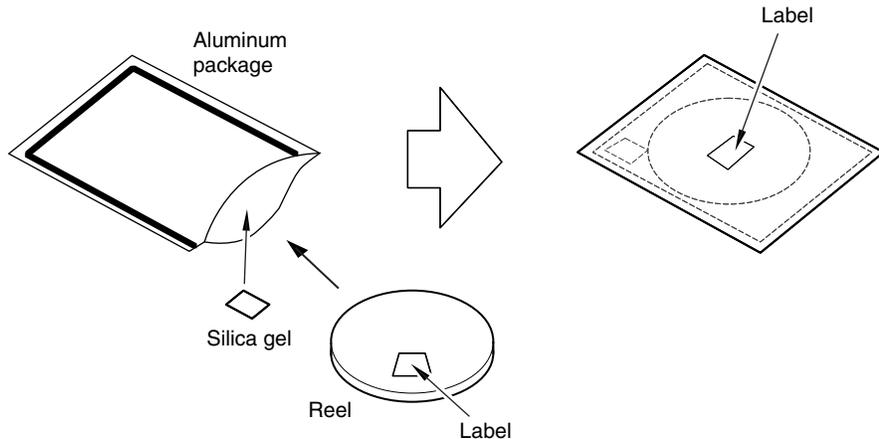
2. Store these parts between 5°C and 30°C, at a relative humidity of less than 60%.
