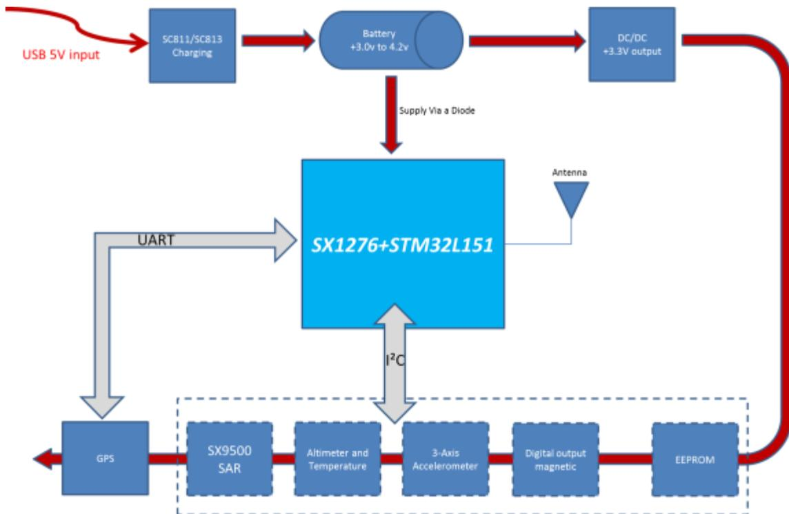
**Figure 2: Block diagram of LoRa sensor node**
