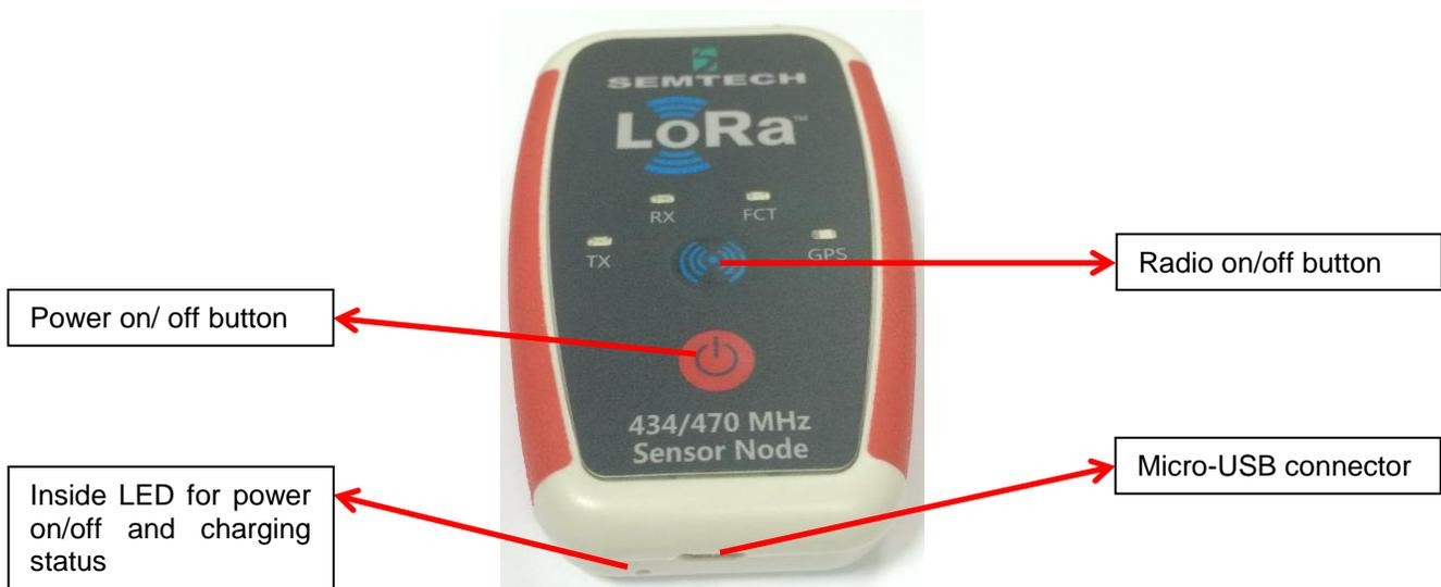
**Figure 1: keyboard and connector of LoRa sensor node**
