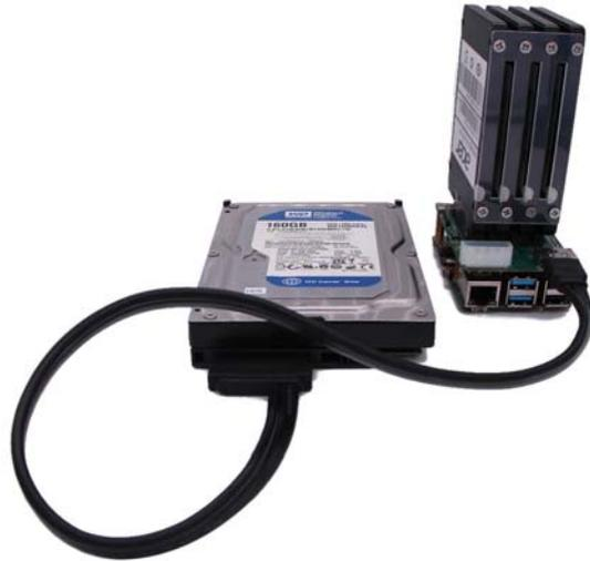
The Penta SATA HAT is powered by the JMB585 with 2 5Gbps PCIe buses with up to 10Gbps bandwidth. With 5 SSD's configured in Raid0 mode, an archiving speed of up to 803MB/s can be achieved.
