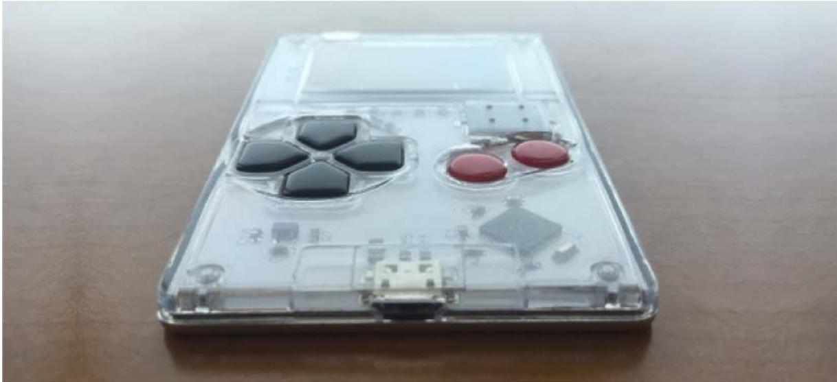
A polycarbonate front, ultra thin circuit board, and stamped metal back gave us the ultimate combination.
