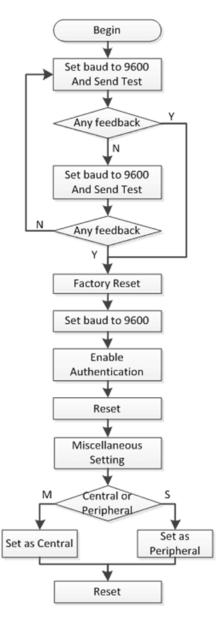
After the initialization, the Central and Peripheral will do different things, the Central will send message to Peripheral interval and print what received from Peripheral while the Peripheral only responds the Central.
