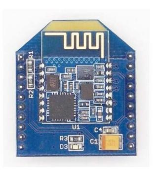
BLE (dual) Bee v1.0 uses CSR dual mode Bluetooth chip, with the ARM architecture single chip which supports AT instructions, Users can develop flexibly according to the serial baud rate, equipment name, pairing password.
