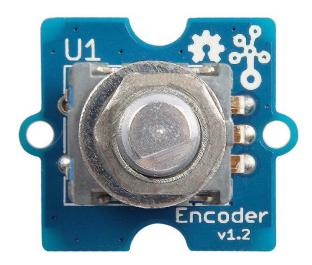
This module is an incremental rotary encoder. It encodes the rotation signal from the axis and output the signal by electronic pulse. The Grove – Encoder is one of the Grove series and has a standard Grove interface. When you need to add a rotary knob to your project, for example a volume knob for a speaker, a selection panel or a digital input, this will be your first choice.
