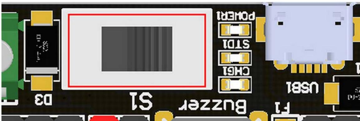
Turn on the switch (in the direction of green terminal input), will provide onboard 3.3V 5V and VM(motors and servos directly driver by battery cell)
