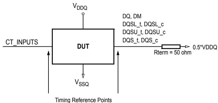
Figure 20. Connectivity Test Mode Timing Reference Load
