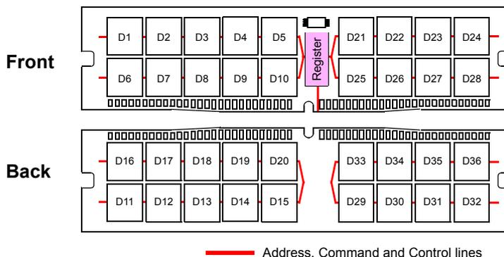
The used device is 4G x4 DDR4 SDRAM, Flip-Chip.
