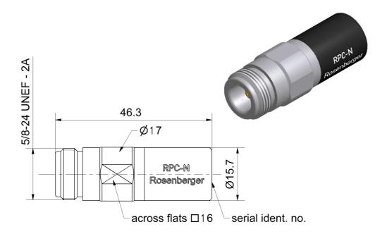
All dimensions are in mm; tolerances according to ISO 2768 m-H
