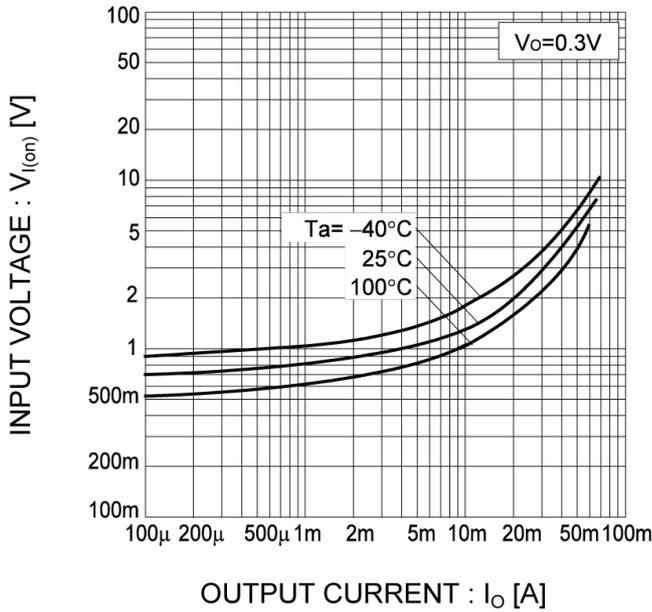
Fig.2 Output Current vs. Input Voltage
