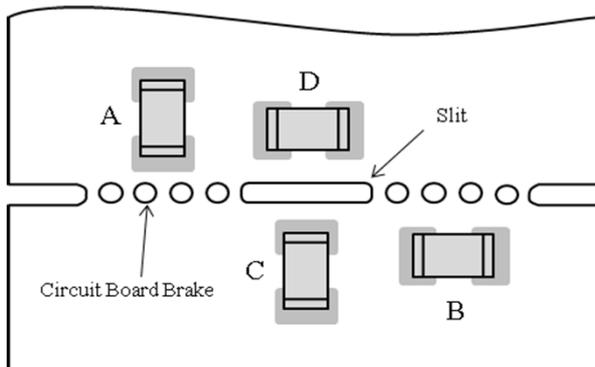
Stress strength according to the mounting position:
