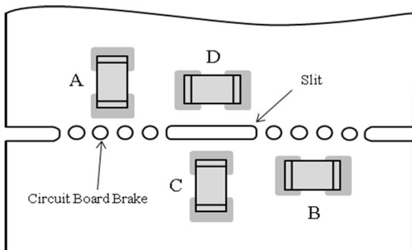
Stress strength according to the mounting position:
