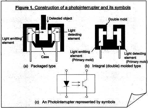
A packaged type photointerrupter, used most commonly, is contained in a molded (injection molded) case, which contains a pair of light emitting and light detecting elements. A double molded type, on the other hand, is a product developed responding to the recent needs of compact-size photointerrupters.
