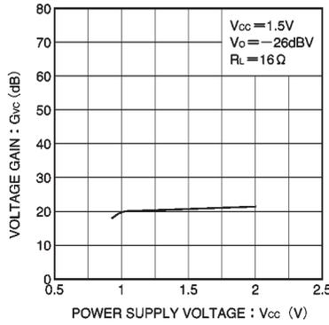
Fig. 14 Voltage gain vs. power supply voltage
