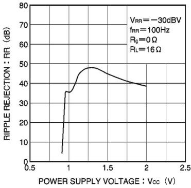
Fig. 13 Ripple rejection ratio vs. power supply voltage
