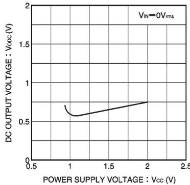
Fig. 11 DC output voltage vs. power supply voltage
