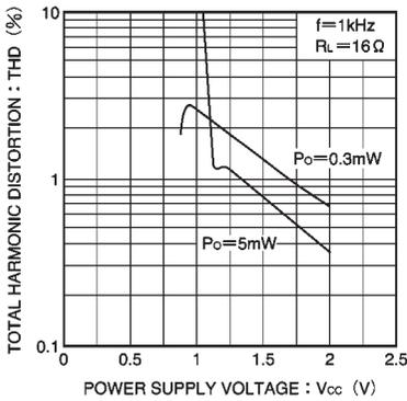
Fig. 16 Total harmonic distortion vs. power supply voltage
