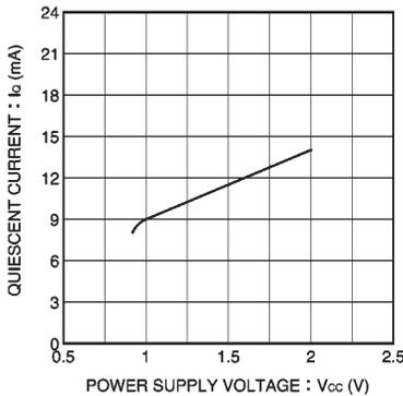
Fig. 10 Quiescent current vs. power supply voltage
