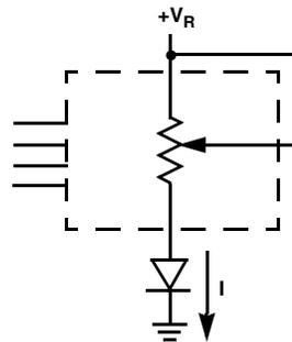
TWO TERMINAL VARIABLE RESISTOR;
