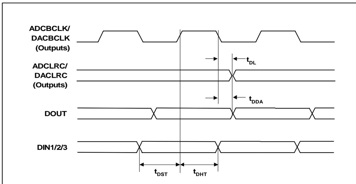
Figure 39 Digital Audio Data Timing – Master Mode
