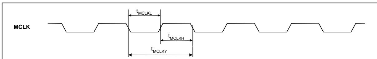
Figure 13 ADC and DAC Master Clock Timing Requirements
