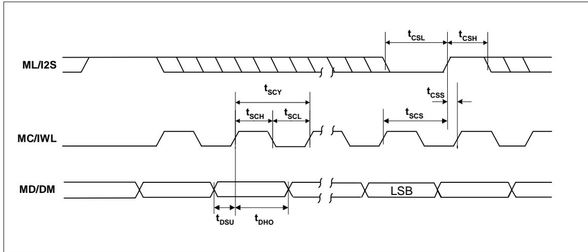
Figure 18 SPI Compatible Control Interface Input Timing
