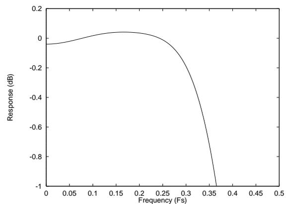
**Figure 4 DAC Digital Filter Ripple – 192kHz**
