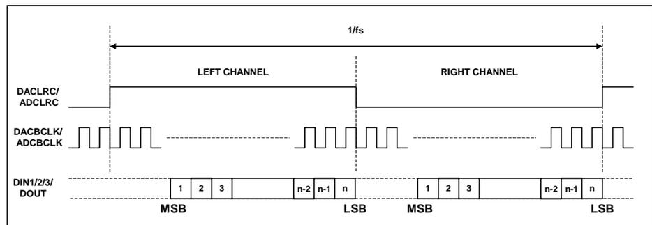
Figure 48 Right Justified Mode Timing Diagram
