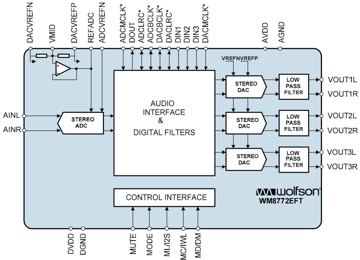
\* extra pins on TQFP allow separate clocking of ADC and DAC
