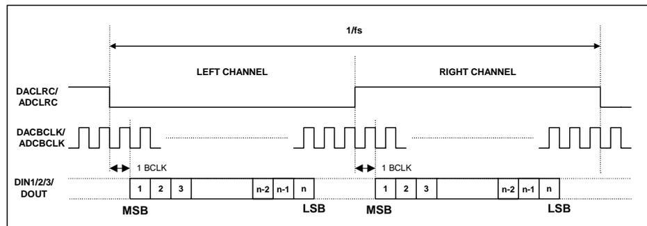
Figure 25 I<sup>2</sup>S Mode Timing Diagram
