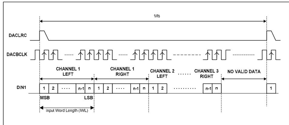
Figure 54 DSP Mode Audio Interface - Mode B Slave, DAC
