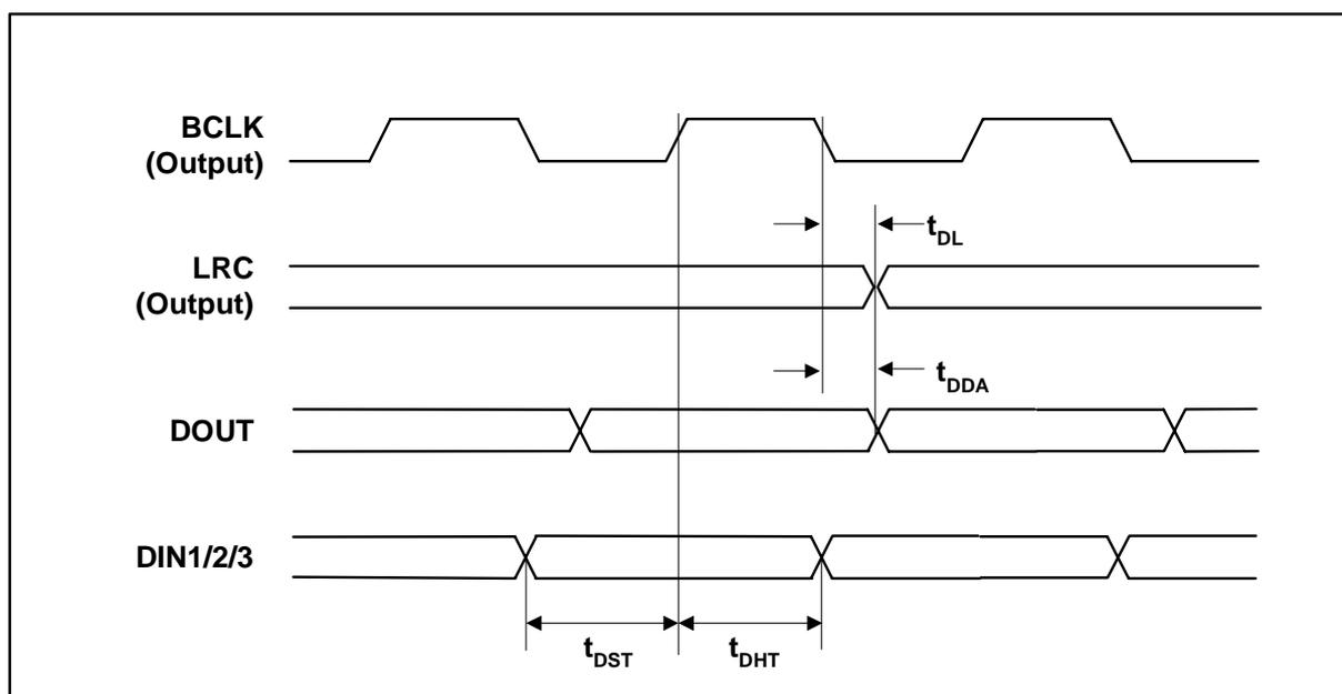
Figure 15 Digital Audio Data Timing – Master Mode
