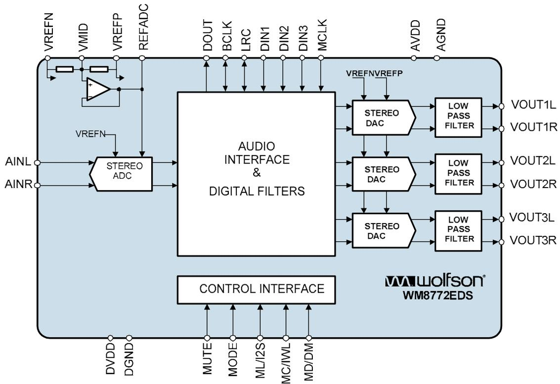
**BLOCK DIAGRAM – 32 LEAD TQFP**
