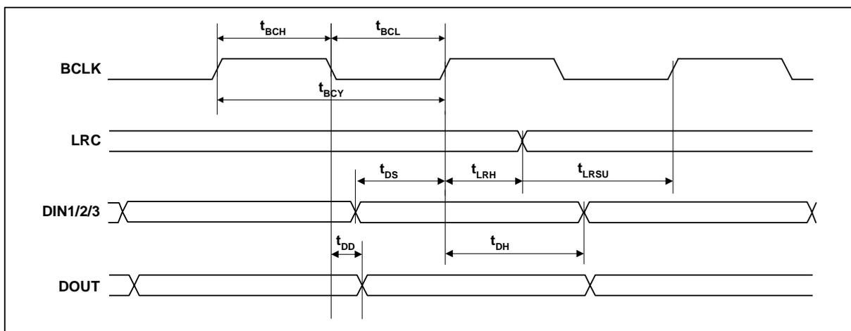
Figure 17 Digital Audio Data Timing – Slave Mode
