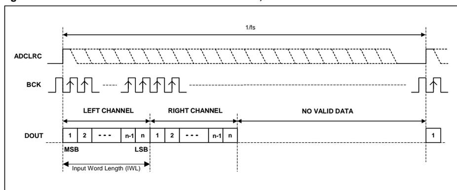
Figure 33 DSP Mode Audio Interface - Mode B Master, ADC
