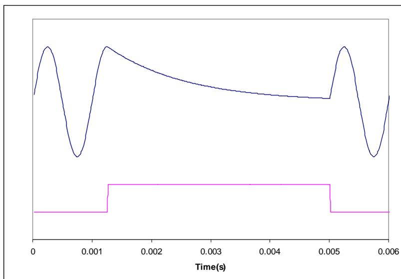
Figure 43 Application and Release of Soft Mute
