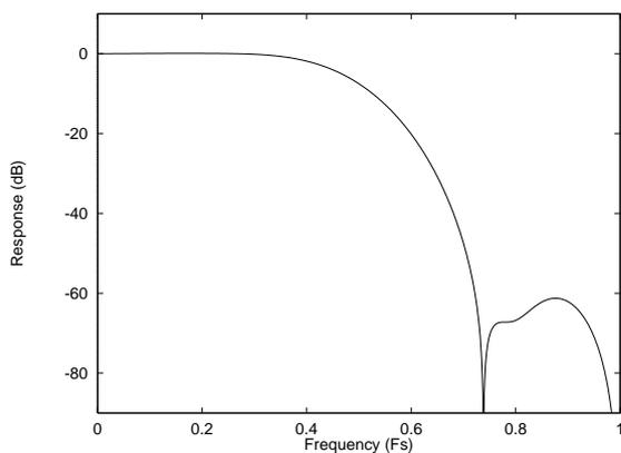
**Figure 3 DAC Digital Filter Frequency Response – 192KHz**
