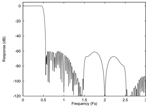
**Figure 1 DAC Digital Filter Frequency Response – 44.1, 48 and 96KHz**
