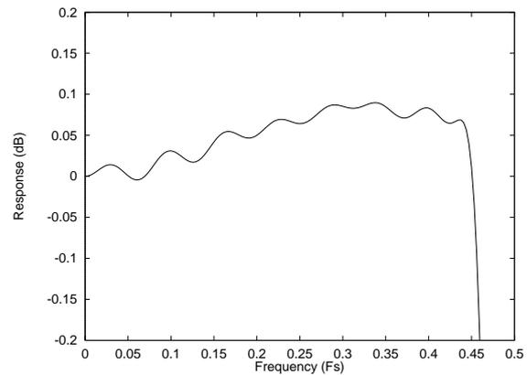
**Figure 2 DAC Digital Filter Ripple –44.1, 48 and 96kHz**
