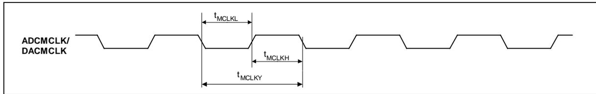
Figure 37 ADC and DAC Master Clock Timing Requirements
