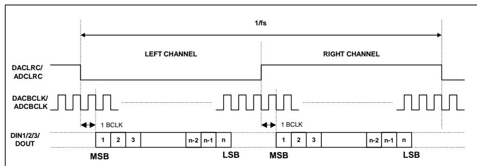
Figure 49 I<sup>2</sup>S Mode Timing Diagram
