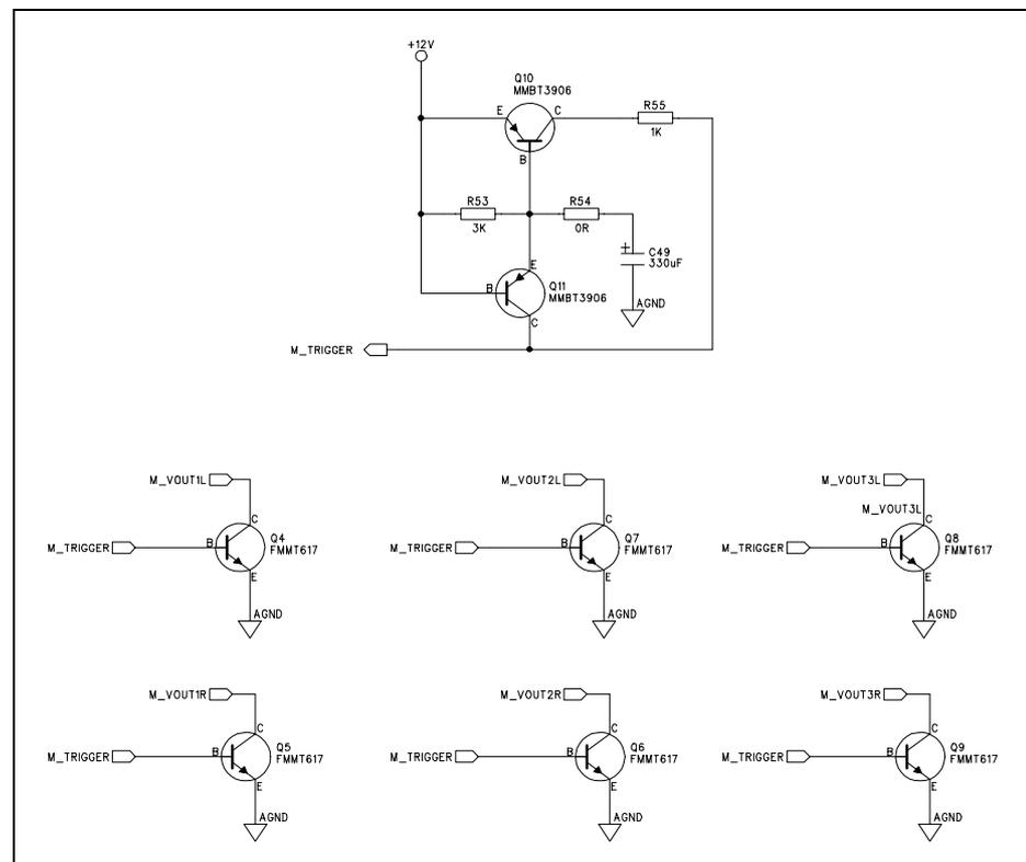
**Figure 36 Output Clamp Circuit**
