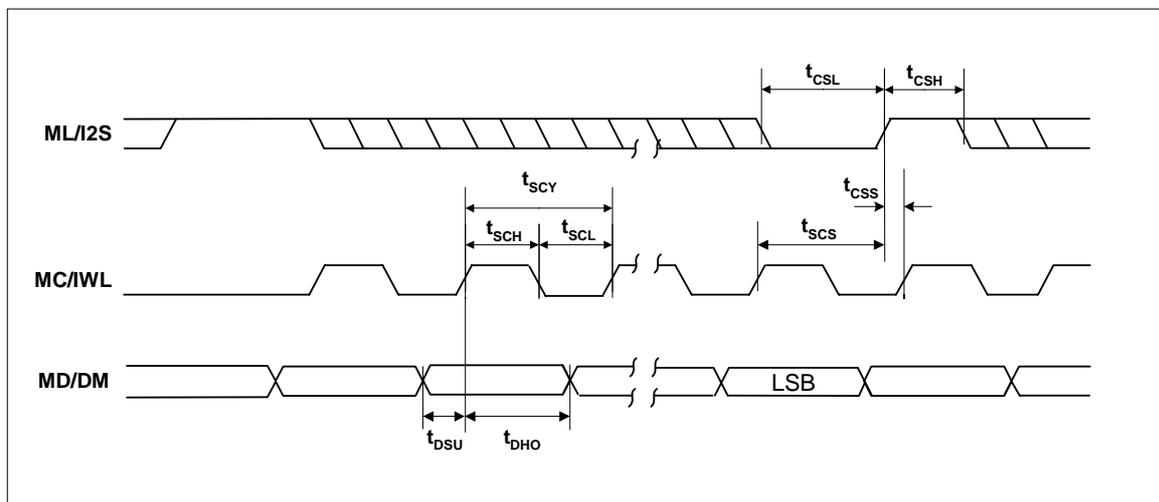
Figure 42 SPI Compatible Control Interface Input Timing
