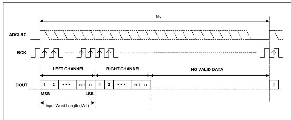
Figure 57 DSP Mode Audio Interface - Mode B Master, ADC
