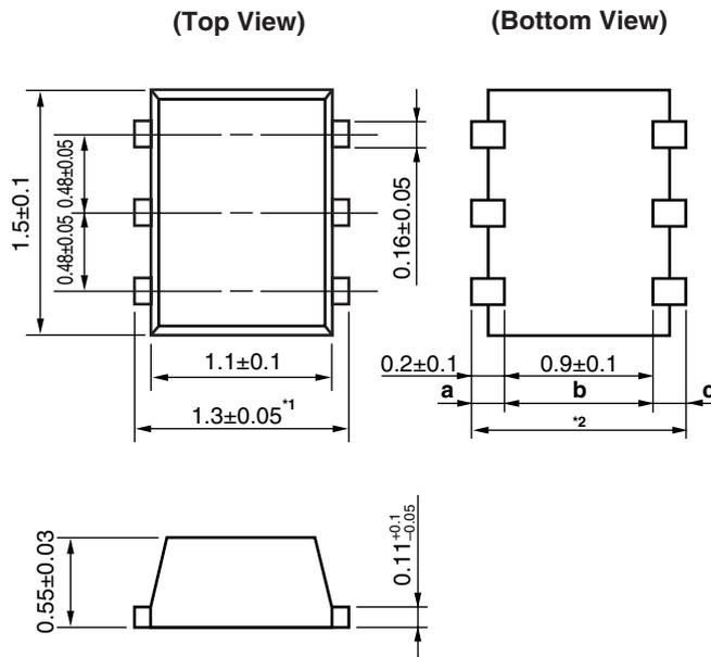
**Remark** Dimension <sup>\*1</sup> is bigger than dimension <sup>\*2</sup> (dimension <sup>\*2</sup> = a + b + c).
