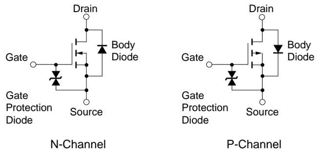
**Remark** The diode connected between the gate and source of the transistor serves as a protector against ESD. When this device actually used, an additional protection circuit is externally required if a voltage exceeding the rated voltage may be applied to this device.
