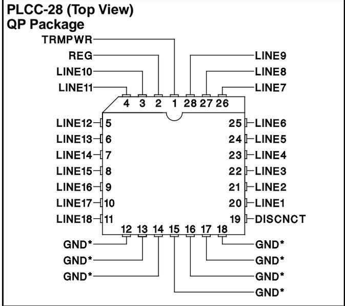
\* QP package pins 12 - 18 serve as both heatsink and signal ground.
