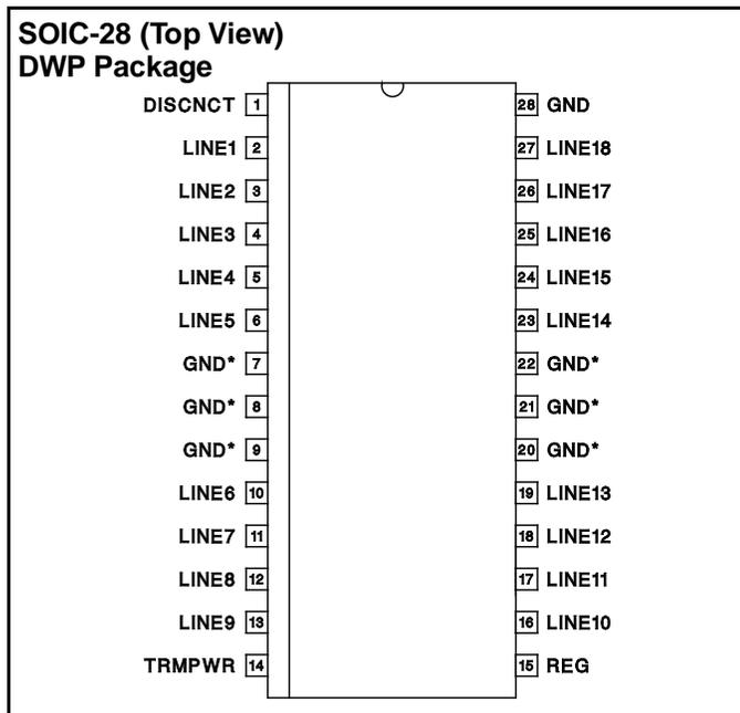
\* DWP package pin 28 serves as signal ground; pins 7, 8, 9, 20, 21, 22 serve as heatsink/ground.
