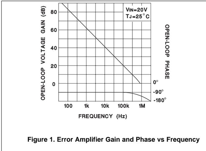
Figure 1. Error Amplifier Gain and Phase vs Frequency
