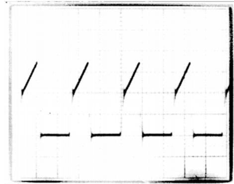
Figure 11. Switch Current Showing Flux Balance in UCX846/7
