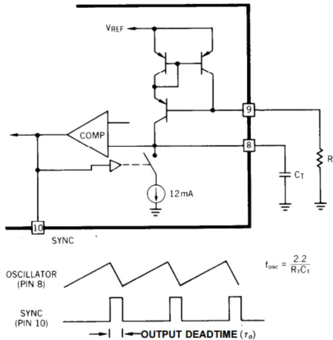
Figure 4. Oscillator Circuit
