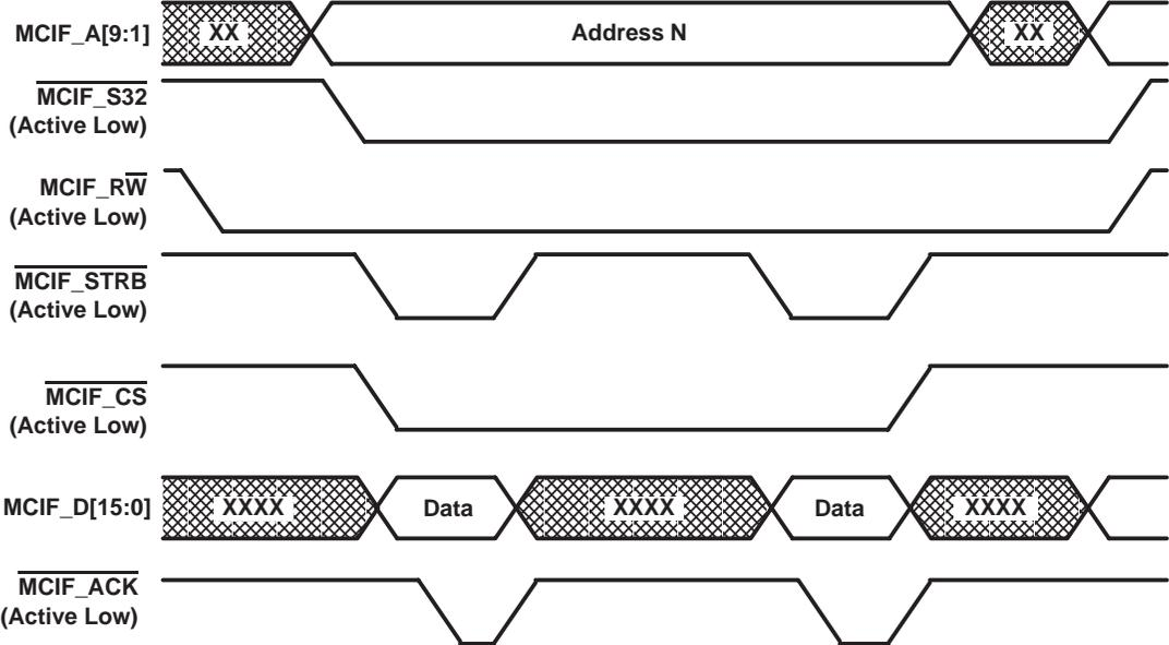
NOTE:  $\overline{\text{MCIF\_CS}}$  can be deasserted between the data phases of a 32-bit access. The  $\overline{\text{MCIF\_STRB}}$  signal acts as the master enable for MCIF.
