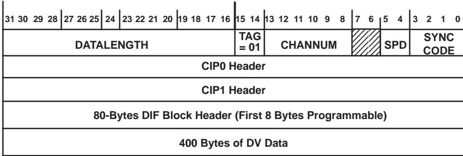
Figure 5–19. DV Transmit Format – DIF Sequence
