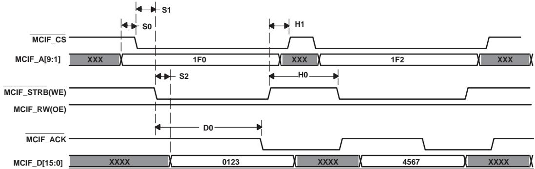
Figure 3–11. Multistrobe Mode – Write Critical Timing
