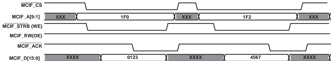
**Figure 3–9. Host Port Multistrobe Timing – Write Operation**
