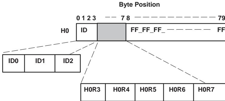
**Figure 5–23. H0 DIF Block Header for DV Transmit**
