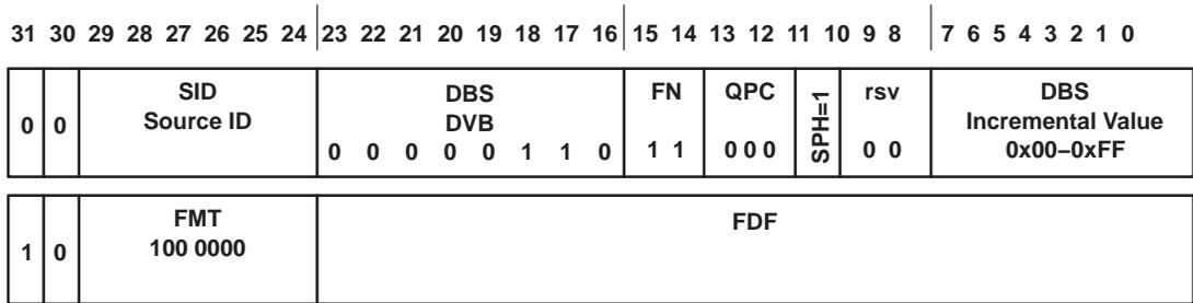
Figure 5–13. Isochronous CIP Headers – MPEG2 Data
