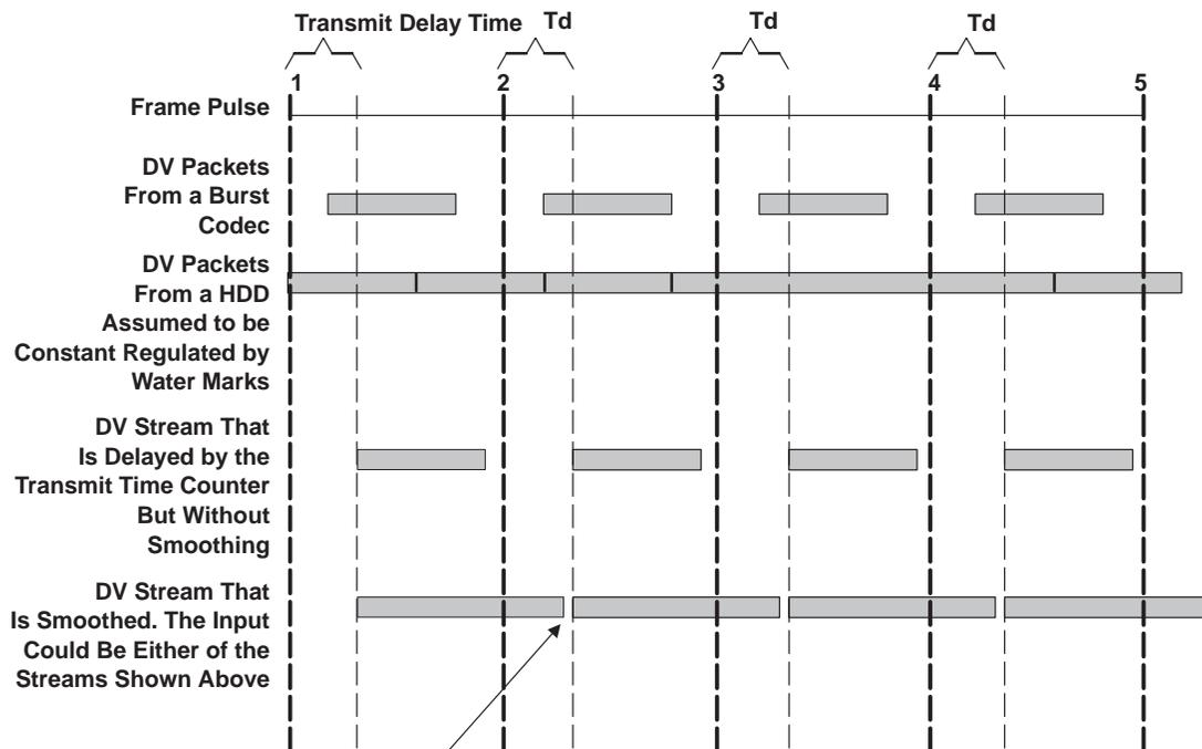
When an ISO cycle occurs during this gap an empty packet will be inserted. It is possible for up to two empty packets to occur during this gap.
