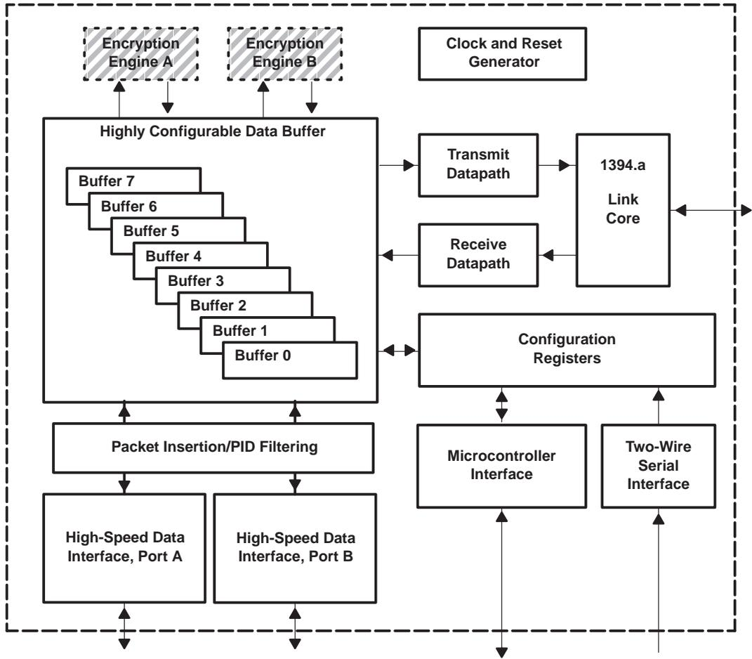
† Shaded region (encryption engines A and B) are only implemented in TSB42AA4.
