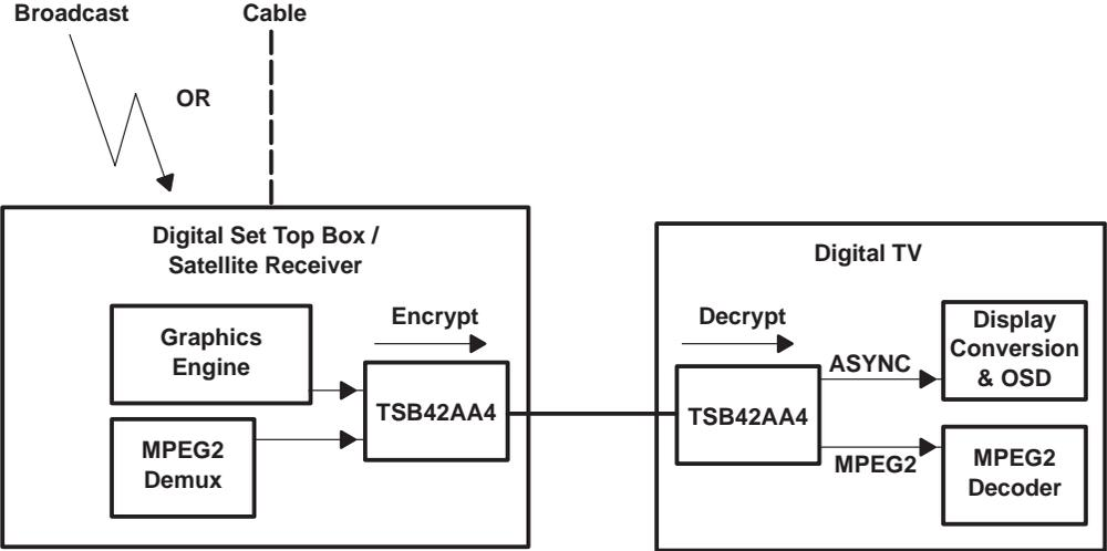
Figure 2-2. Graphics Overlay From Digital STB to DTV
