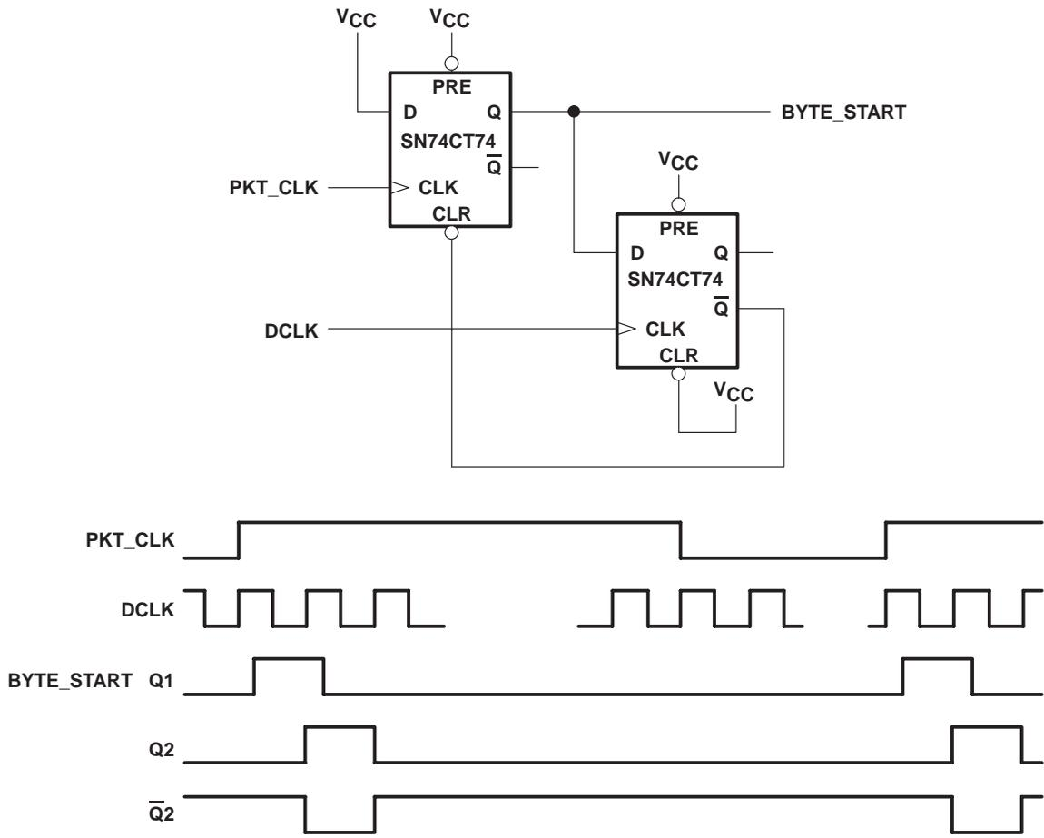
**Figure 3–23. Typical Byte Start Circuit**
