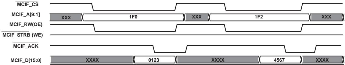
Figure 3–10. Host Port Multistrobe Timing – Read Operation
