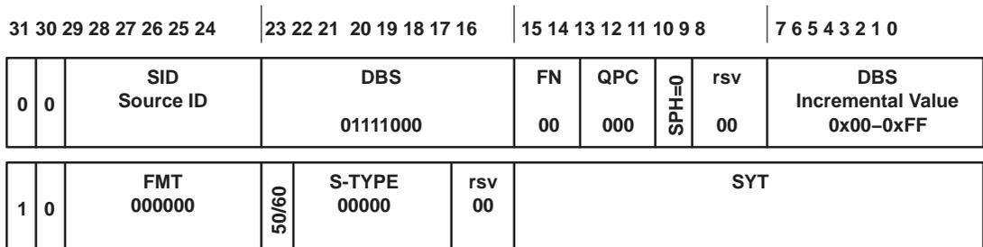
Figure 5–22. Isochronous CIP Headers – DV Data
