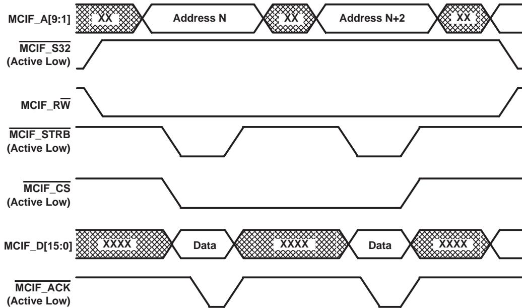
NOTE: MCIF\_CS can be deasserted between the two 16-bit transactions. The MCIF\_STRB signal acts as the master enable for MCIF.
