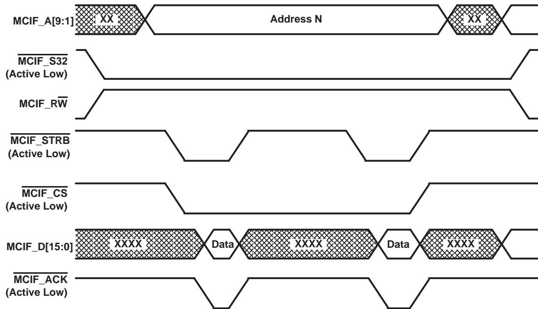
NOTE:  $\overline{\text{MCIF\_CS}}$  can be deasserted between data phases of 32-bit read. The  $\overline{\text{MCIF\_STRB}}$  acts as the master enable for the MCIF.
