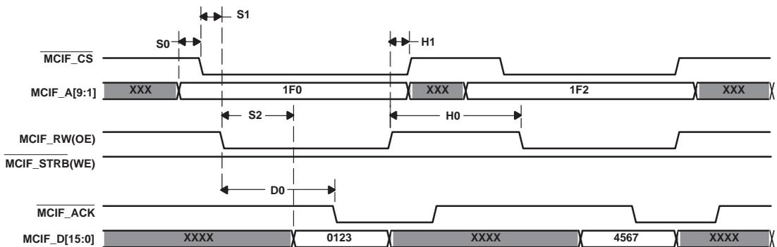
Figure 3–12. Multistrobe Mode – Read Critical Timing
