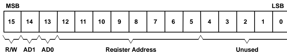
Figure 5. Bit Assignment and Definition for Slot-0 Word
